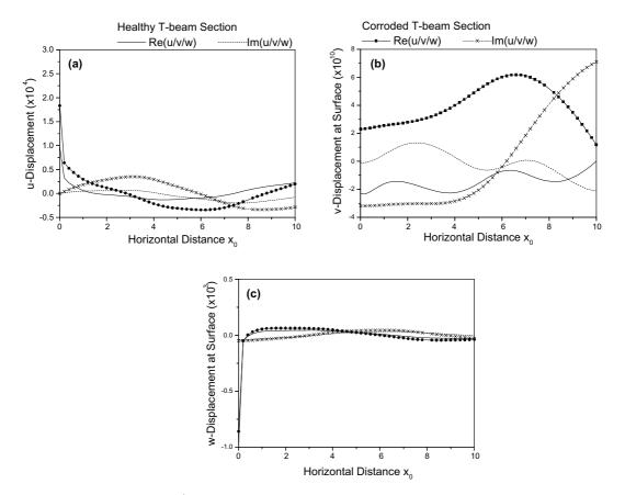
Fig. 7. Surface displacements at  $y = W_f/2$  for reinforced T-beam (and reinforced T-beam with 10% corrosion of steel) along the top surface of the beam at  $\Omega = 1$ .
