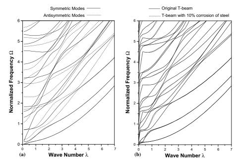
Fig. 5. Dispersion curves for (a) unreinforced and (b) reinforced T-beam (original and with 10% corrosion of steel).
