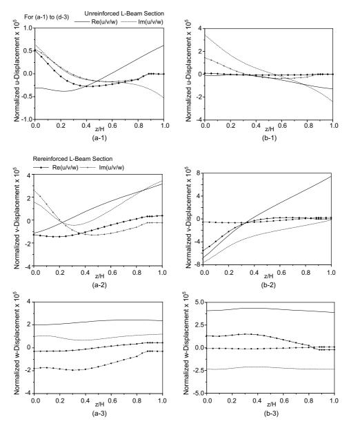
Fig. 9. Displacements u, v, w along thickness direction and at y = 0.3H for unreinforced L-beam at section (a) x = 0.2H,  $\Omega = 1$ ; (b) x = 10H,  $\Omega = 1$ ; and for reinforced L-beam (and reinforced L-beam with 10% corrosion of steel) at section (c) x = 0.2H,  $\Omega = 1$ ; (d) x = 10H,  $\Omega = 1$ .
