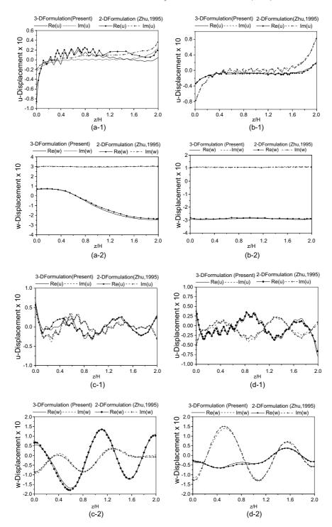
Fig. 3. The normalized horizontal and vertical displacements (u, w) for a 35 layer graphite epoxy plate at section (a) x = 0.2H,  $\Omega = 1$ ; (b) x = 10H,  $\Omega = 1$ ; (c) x = 0.2H,  $\Omega = 10$  and (d) x = 10H,  $\Omega = 10$ .
