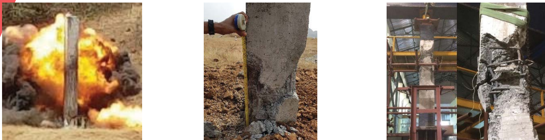
a) Contact blast b) post-blast damage c) Residual axial capacity test Figure 5: Field trial for blast performance and residual capacity test of RC column
