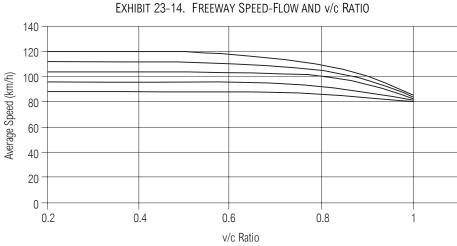
For a rural freeway, the capacity per lane is 2,400 pc/h/ln, based on the assumption that rural freeways have interchange spacing of greater than 3.0 km and two lanes in one direction. Exhibit 23-15 can be used to determine capacity for urban freeways with shorter interchange spacing or a different number of lanes.
