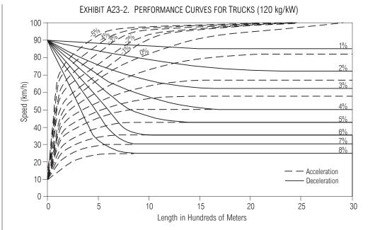
The composite grade procedure is not applicable in all cases, especially if the first segment is downgrade and the segment length is long, or the segments are too short. In using the performance curves, cases that cannot be solved with this procedure will become apparent to the analyst because lines will not intersect or points will fall outside the limits of the curves. In such cases, field measurement of speeds should be used as input to the selection of appropriate truck equivalency values.
