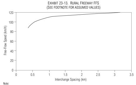
Assumptions: BFFS = 120 km/h, lane width = 3.6 m, lateral clearance = 1.8 m.
