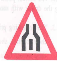
Divided Road Ends
