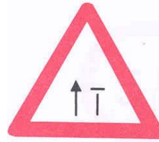
Lane Closed (Two Lane Road)
