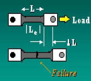
failure strain ( $r_f$ ) =  $\frac{c \text{ hange in length ($L$)}}{effective gauge length ($L_o$)}$
