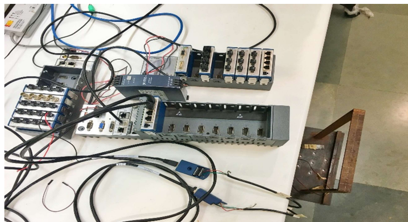
National Instruments Compact Rio DAQ (Multifunctional- Acceleration, Strains, Voltage, Temperature Sensing)
