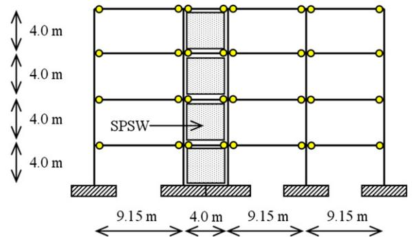
Fig. 3. Configuration of the study frame with an SPSW.
