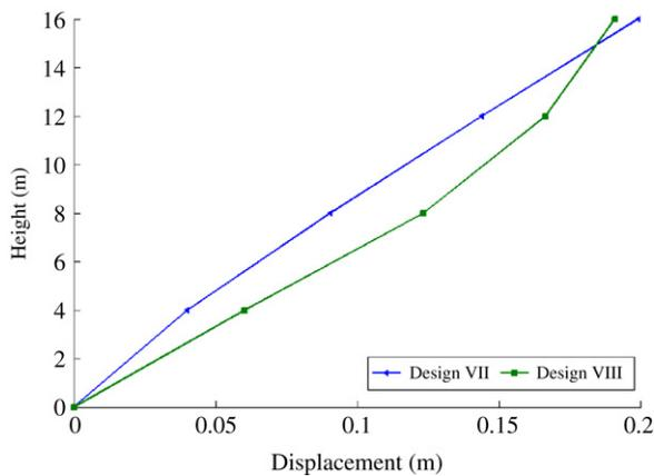
**Fig. 5.** Displacement profiles at peak roof displacement for Designs VII and VIII.
