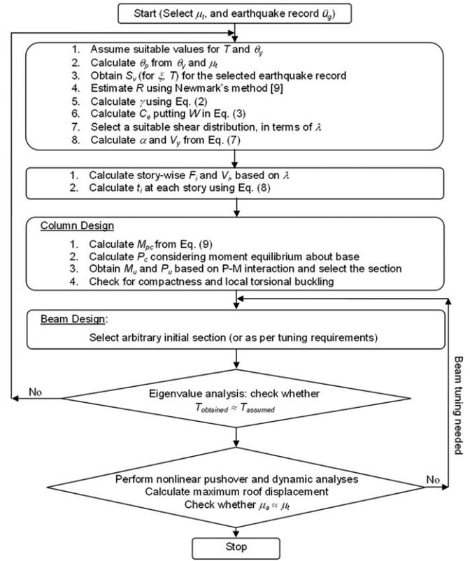
Fig. 2. Flowchart for the proposed design method.
