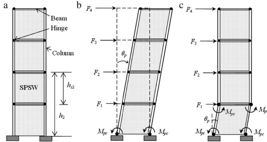
Fig. 1. (a) Schematic of the SPSW system; (b) Selected yield mechanism; (c) Soft ground story.
