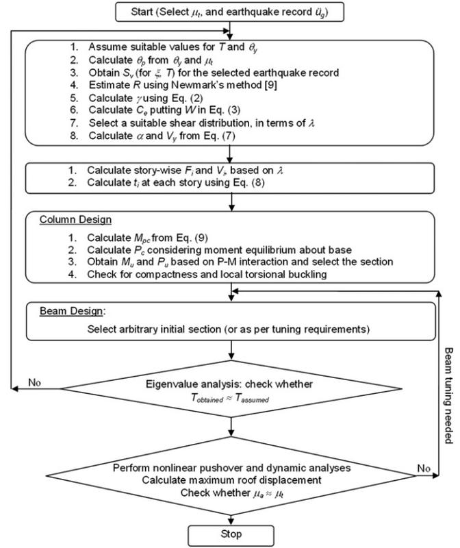
Fig. 2. Flowchart for the proposed design method.
