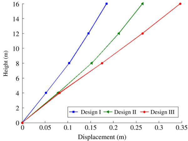
**Fig. 4.** Displacement profiles at peak roof displacement for Designs I, II and III.
