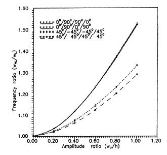
**Figure 5**. Variation of frequency ratio  $(w_{NL}/w_L)$  of a square cross-stiffened composite plate with amplitude ratio  $(w_0/h)$  for five different ply orientations (Case 3).
