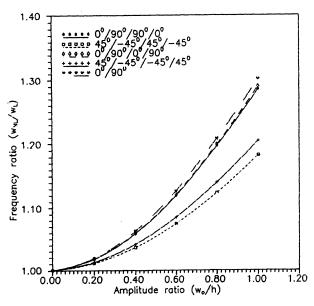
**Figure 3**. Variation of frequency ratio  $(w_{NL}/w_L)$  a square cross-stiffened composite plate with amplitude ratio  $(w_0/h)$  for five different ply orientations (Case 1).
