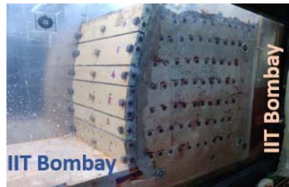
Front elevation of GRSW constructed with marginal backfill subjected to rainfall at 40 g
