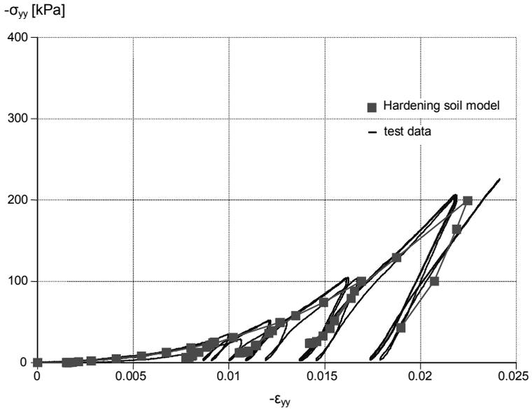
Figure 10.11 Results of oedometer test on loose Hostun sand, axial stress versus axial strain
