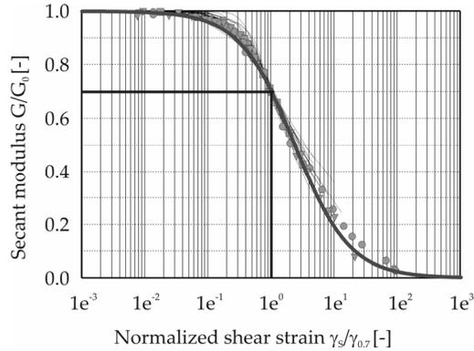
Figure 6.2 Results from the Hardin-Drnevich relationship compared to test data by Santos & Correia [52]
