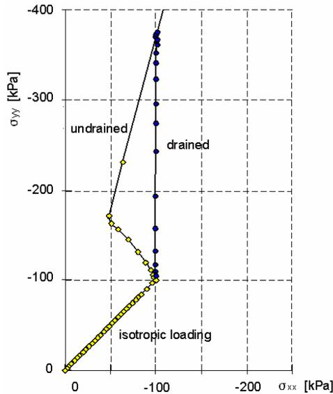
Figure 10.6 Stress paths for drained and undrained triaxial tests using the HS model
