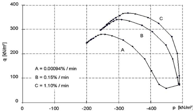
Figure 10.21  $p$ - $q$  stress paths for different rates of straining for a point at position (0.01 , 0.01)
