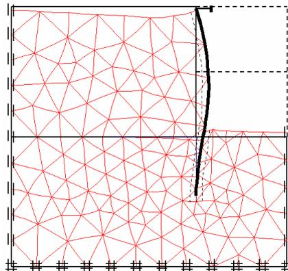
Figure 10.28 Deformed mesh after excavation
