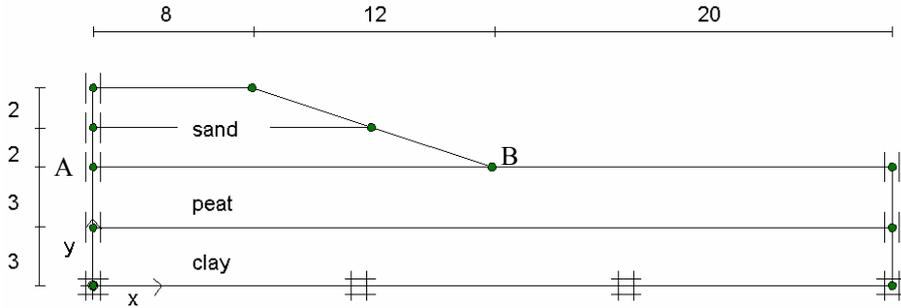
Figure 10.32 Geometry model of road embankment project
