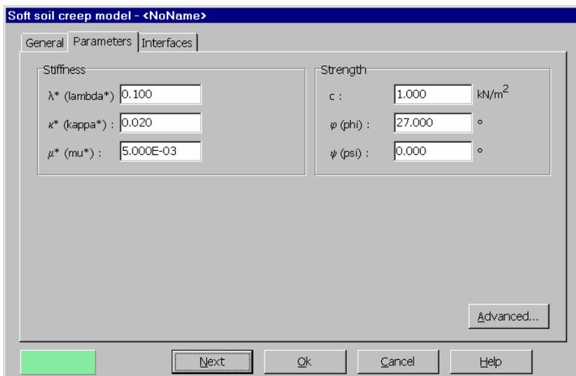
Figure 7.4 Parameters tab sheet for the Soft Soil Creep model
