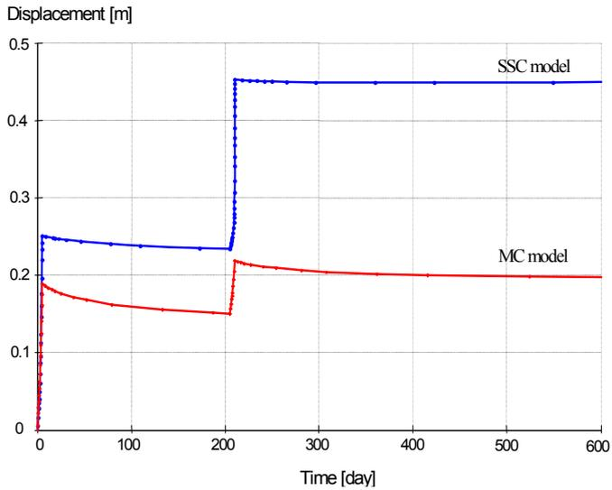
Figure 10.35 SSC model vs. MC model - horizontal displacements at B.
