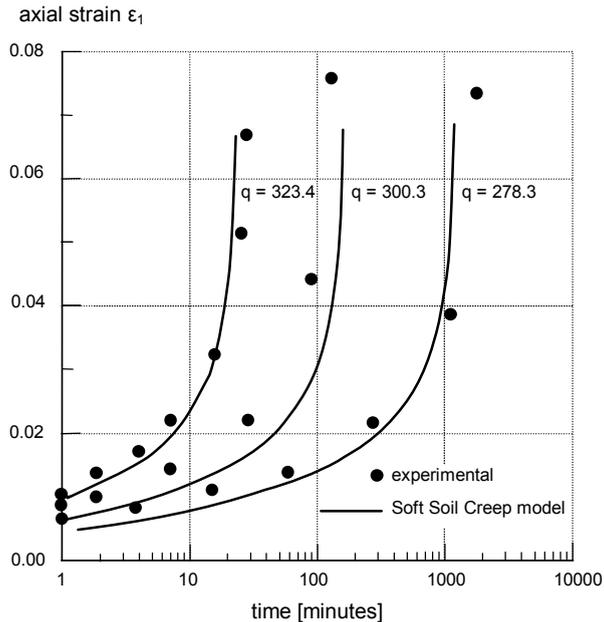
Figure 7.8 Results of triaxial creep tests.
