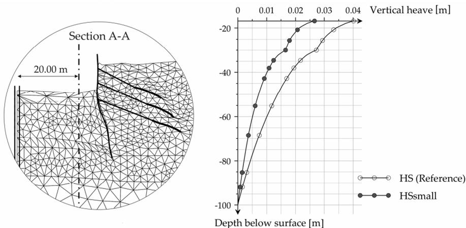
Figure 10.31 Vertical displacements in the excavation pit at a distance of 10 m from the retaining wall (Section A-A).
