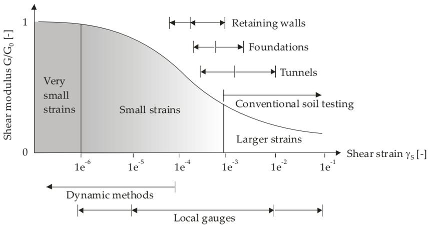
Figure 6.1 Characteristic stiffness-strain behavior of soil with typical strain ranges for laboratory tests and structures (after Atkinson & Sallfors [47])
