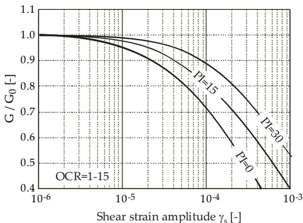
Figure 6.7 Influence of plasticity index (PI) on stiffness reduction after Vucetic & Dobry [54].
