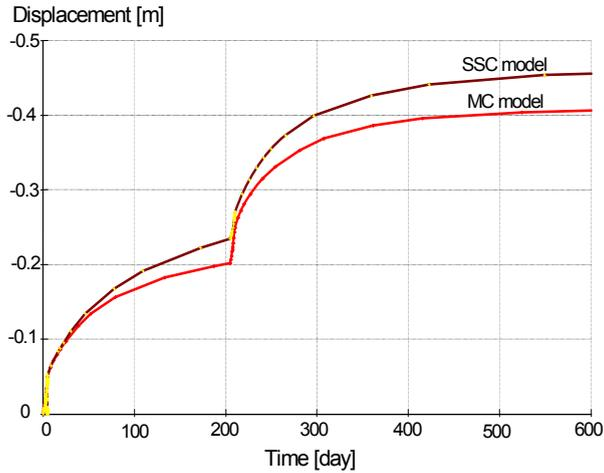
Figure 10.34 SSC model vs. MC model - vertical displacements at A
