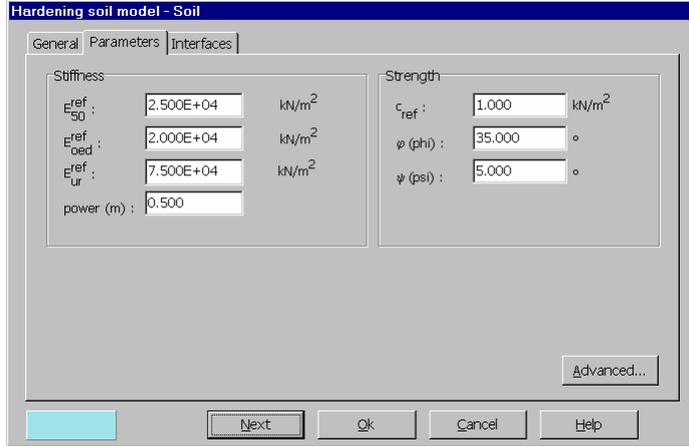
Figure 5.3 Basic parameters tab sheet for the Hardening Soil model
