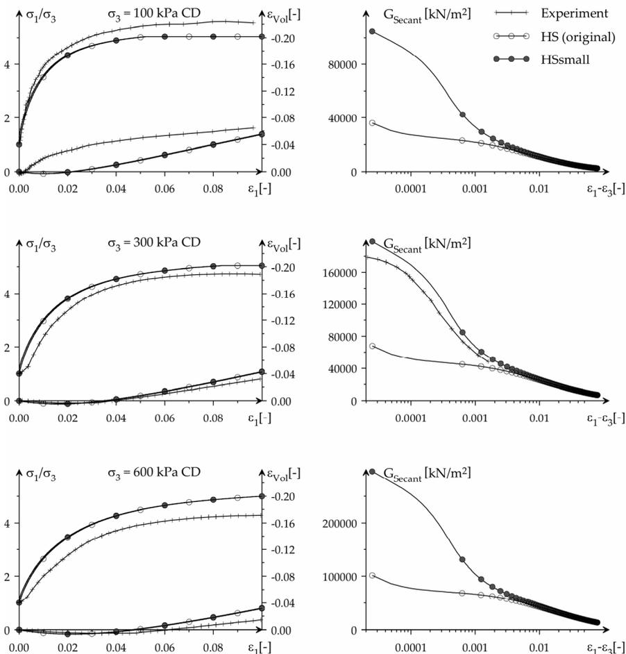
Figure 10.17 Drained triaxial tests on dense Hostun sand at confining pressures of 100, 300, and 600 kPa. Left: Stress-strain data. Right: Shear modulus reduction.
