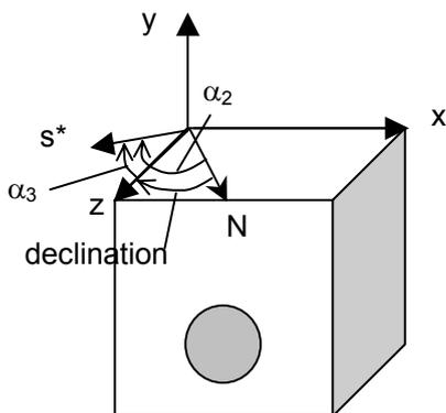
Figure 4.6 Definition of various directions and angles in the horizontal plane
