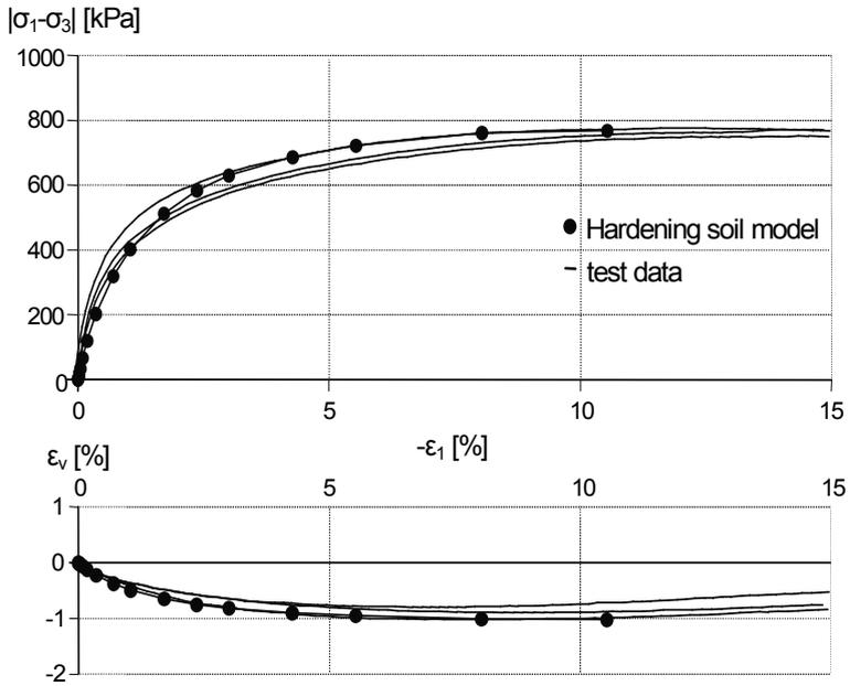
Figure 10.7 Results of drained triaxial tests on loose Hostun sand, principal stress ratio versus axial strain
