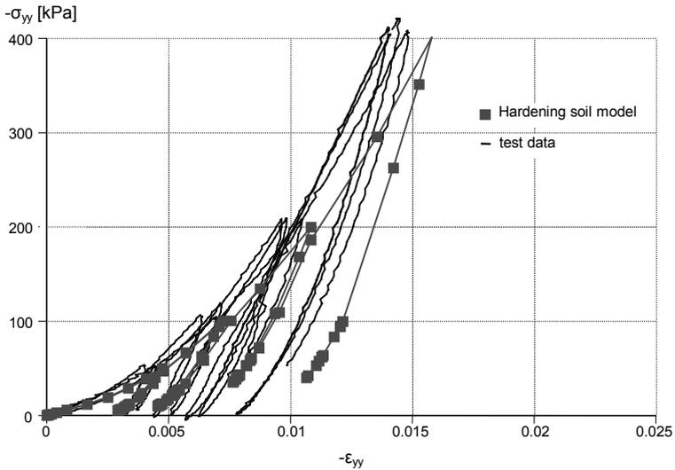
Figure 10.12 Results of oedometer test on dense Hostun sand, axial stress versus axial strain
