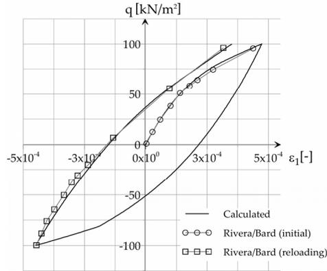
Figure 10.18 Hysteresis loop in a drained triaxial test on dense Hostun sand. Test data published in Biarez & Hicher [55].
