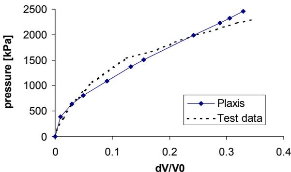
Figure 10.15 Comparison of numerical results and pressiometer test data
