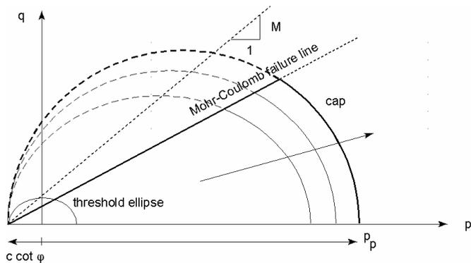
Figure 8.2 Yield surface of the Soft Soil model in  $p'$ - $q$ -plane
