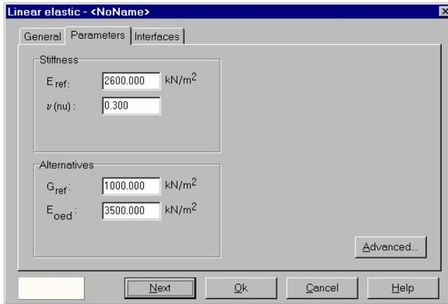
Figure 2.3 Parameters tab for the Linear Elastic model
