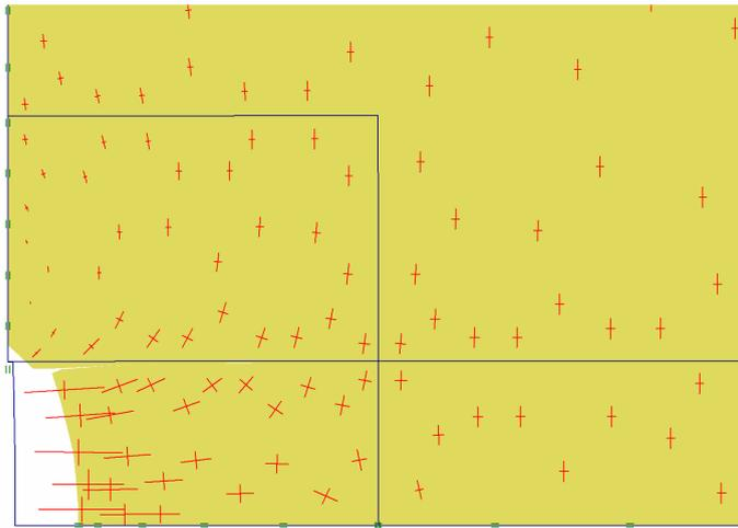
Figure 10.14 Stress distribution in deformed geometry around the pressiometer at a pressure of 2350 kPa
