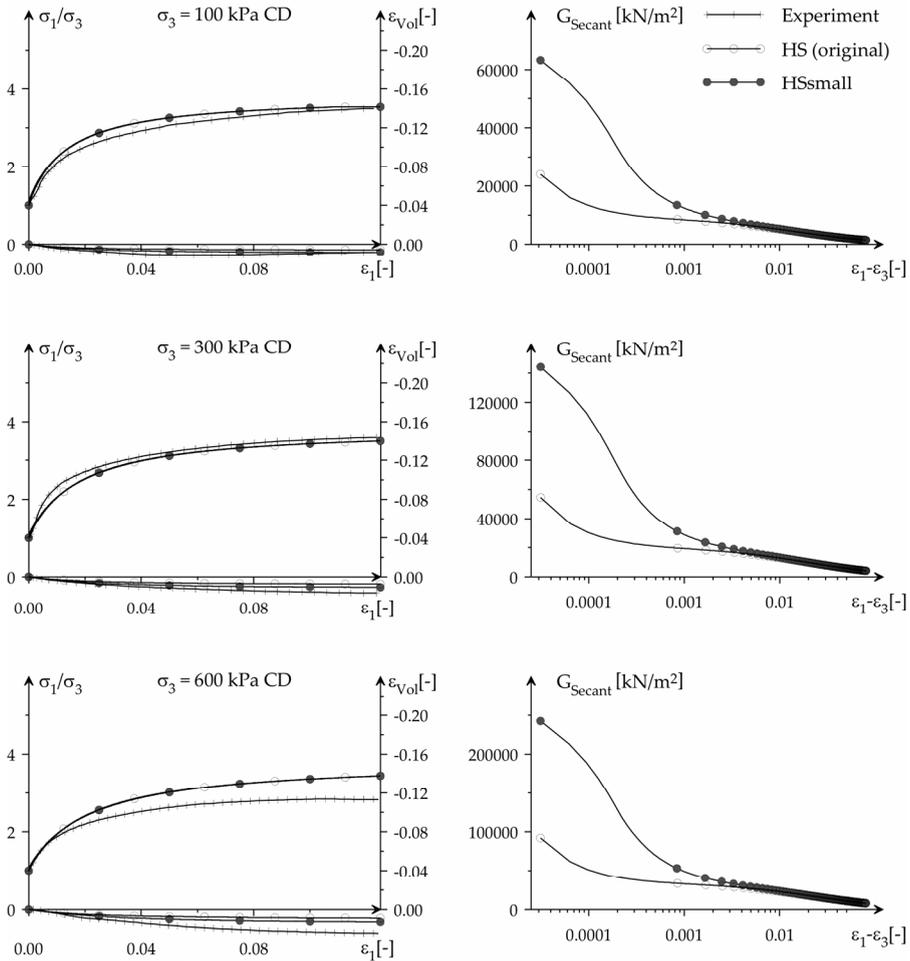
Figure 10.16 Excavation Drained triaxial tests on loose Hostun sand at confining pressures of 100, 300, and 600 kPa. Left: Stress-strain data. Right: Shear modulus reduction.
