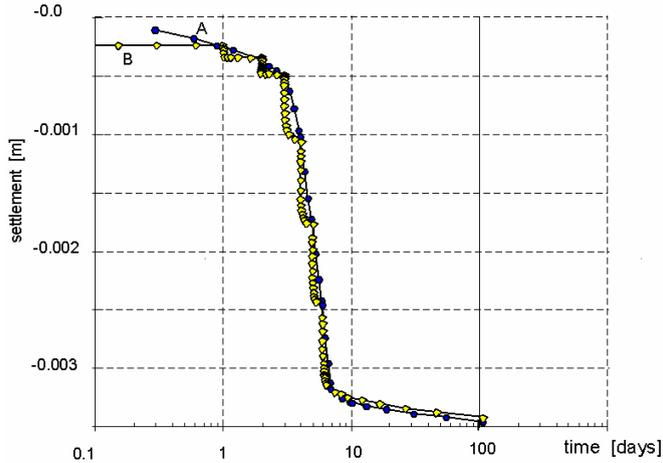
Figure 10.24 Time-settlement curve of oedometer test with Soft Soil Creep model. A) Transient loading with doubling of loading within one day. B) Instantaneous loading with doubling of load at the beginning of a new day
