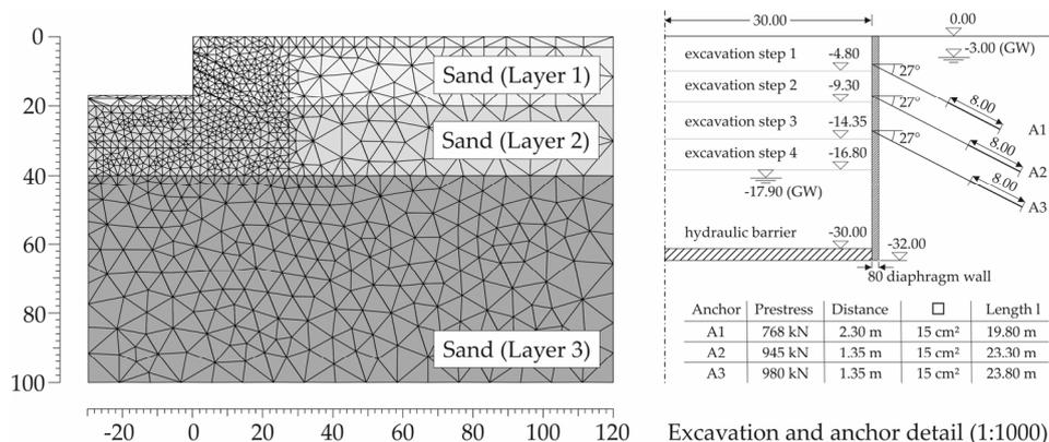
Figure 10.29 Excavation in Berlin sand: plane strain mesh (left) and geometry detail (right).
