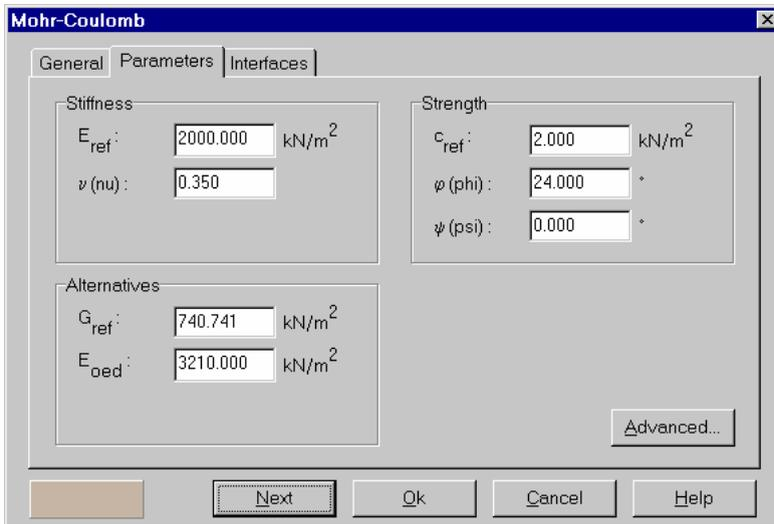
Figure 3.3 Parameter tab sheet for Mohr-Coulomb model
