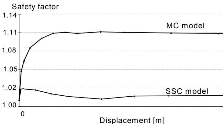
Figure 10.33 Safety factor analysis using MC model and SSC model.
