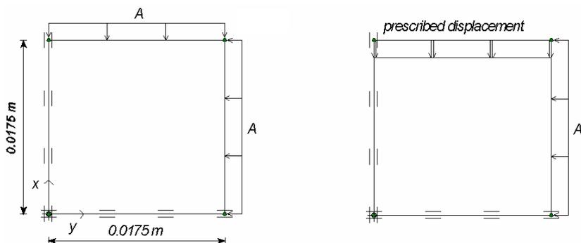
Figure 10.19 Modelling of triaxial test on Haney clay. Left, Initial configuration. Right, configuration for phase 9 - 11
