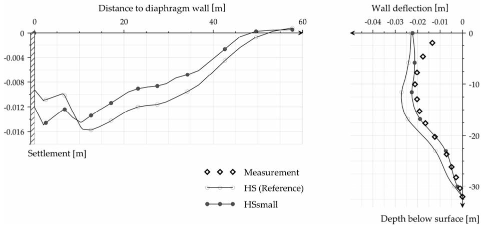
Figure 10.30 HS and HS-Small model predictions versus measured displacements after the final excavation step. Left: Surface settlement trough. Right: Lateral wall deflection.
