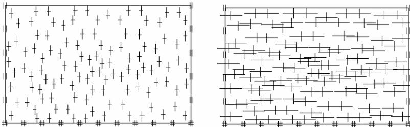
Figure 10.25 Stress states at a vertical stress level of -80 kPa. Left, after primary loading  $\sigma_{xx} \approx -40$  kPa. Right, after unloading from -640 kPa  $\sigma_{xx} \approx -220$  kPa
