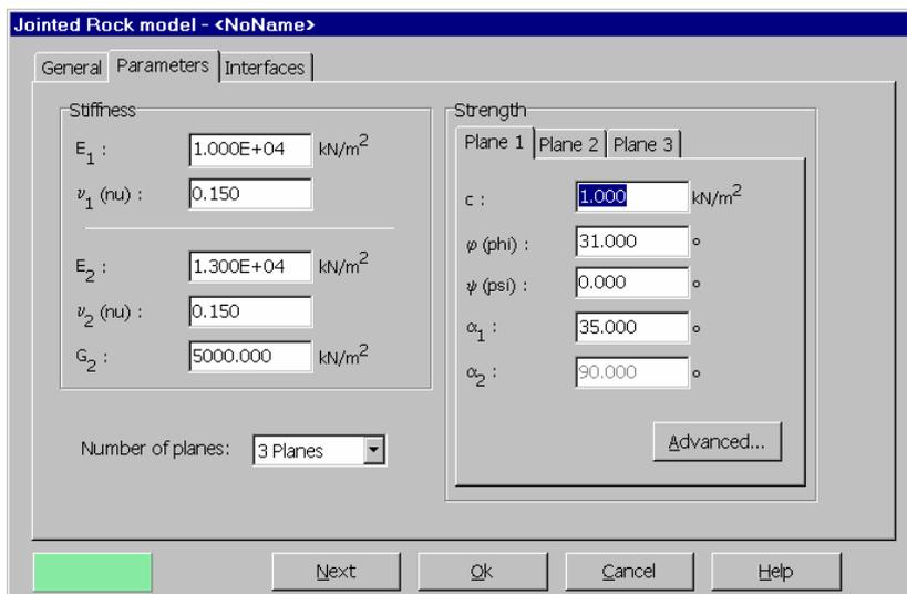
Figure 4.4 Parameters for the Jointed Rock model
