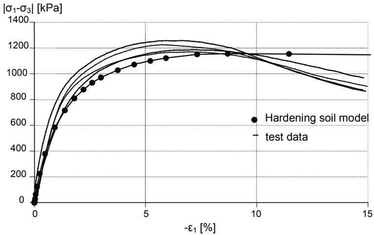
Figure 10.8 Results of drained triaxial tests on dense Hostun sand, principal stress ratio versus axial strain
