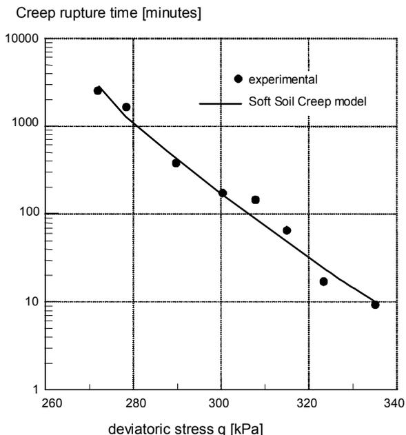
Figure 7.9 Results of triaxial creep tests.
