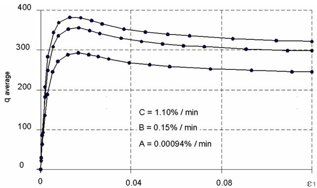
Figure 10.20 Average deviatoric stress versus axial strain for different rates of straining
