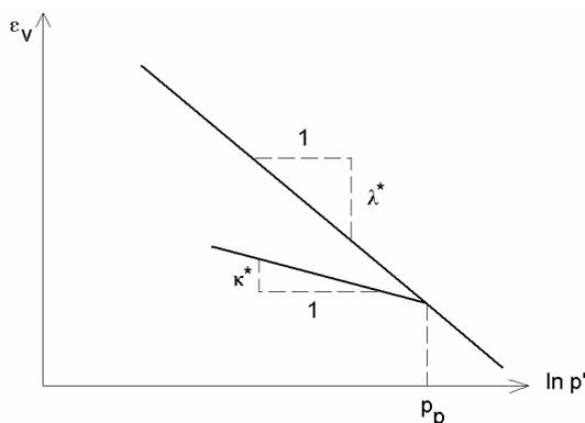
Figure 8.1 Logarithmic relation between volumetric strain and mean stress
