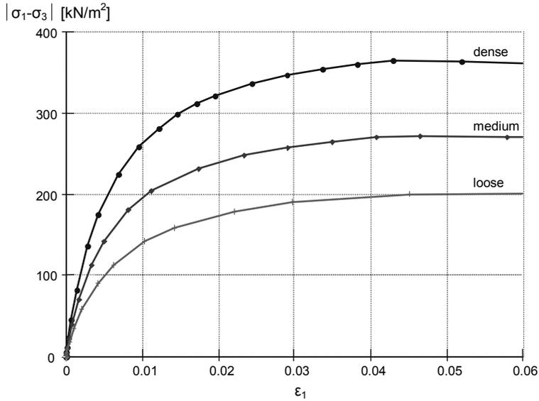
Figure 10.2 Results of drained triaxial tests using the Hardening Soil model, Principal stress difference versus axial strain
