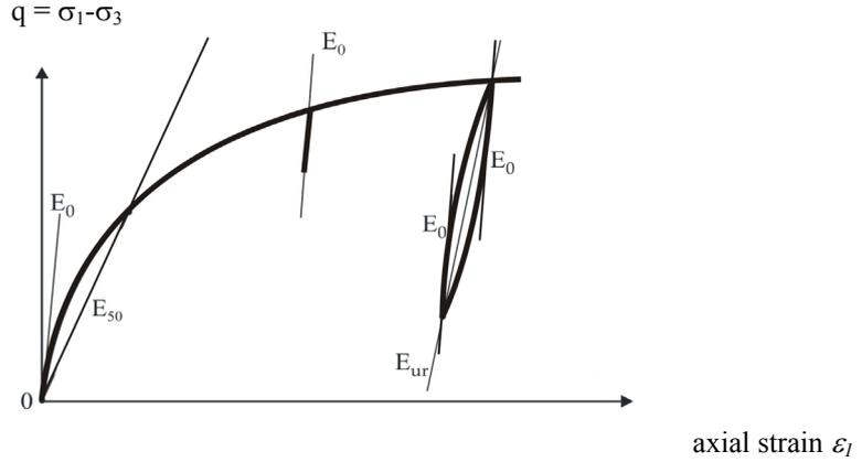
Figure 6.5 Stiffness parameters  $E_{50}$ ,  $E_{ur}$ , and  $E_0 = 2G_0(1 + \nu_{ur})$  of the HSsmall model in a triaxial test
