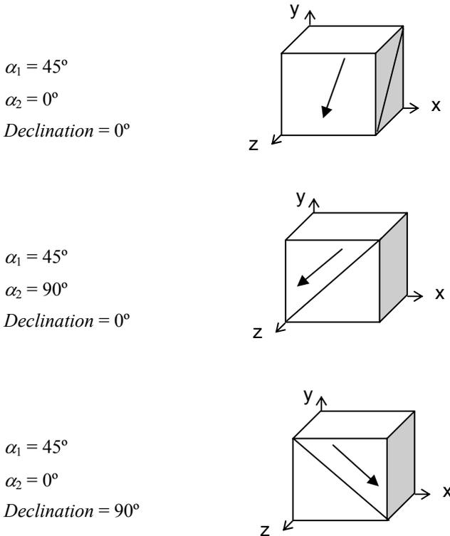
Figure 4.7 Examples of failure directions defined by  $\alpha_1$ ,  $\alpha_2$  and *Declination*
