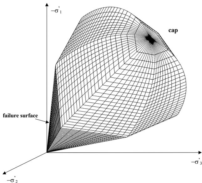
Figure 8.3 Representation of total yield contour of the Soft Soil model in principal stress space
