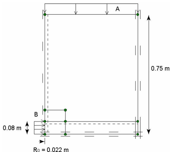
Figure 10.13 Geometry model for pressiometer test
