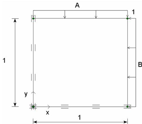
Figure 10.1 Simplified configuration of a triaxial test
