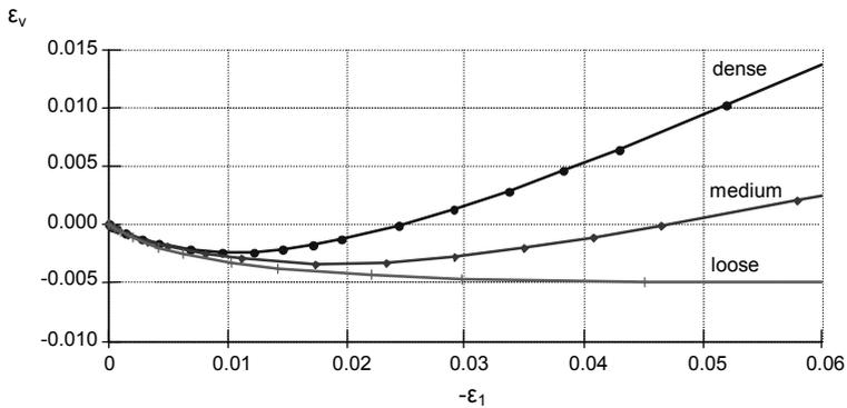
Figure 10.3 Results of drained triaxial tests using the Hardening Soil model, Volumetric strain versus axial strain
