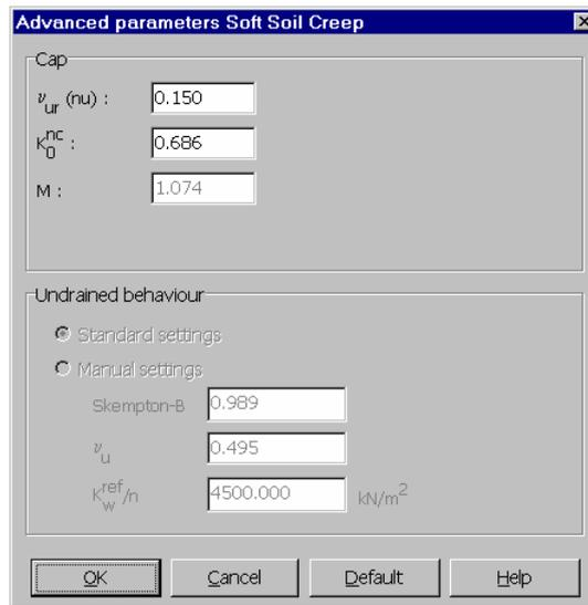
Figure 7.5 Advanced parameters for Soft Soil Creep model
