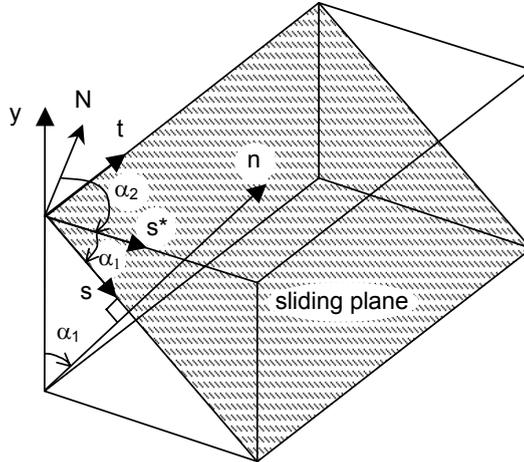
Figure 4.5 Definition of dip angle and dip direction
