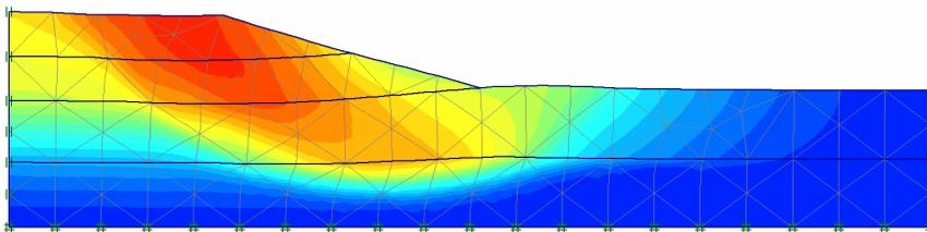
Figure 10.36 Tendency towards failure mechanism after the construction of second part of the embankment
