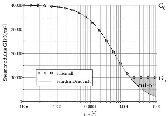
Figure 6.3 Cut-off of the small-strain degradation curve as used in the HS-Small model
