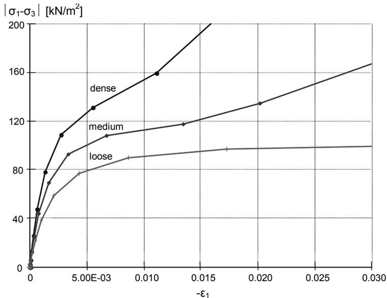
Figure 10.4 Results of undrained triaxial tests using the Hardening Soil model, Principal stress difference versus axial strain
