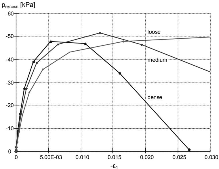
Figure 10.5 Results of undrained triaxial tests using the Hardening Soil model, Excess pore pressure vs axial strain
