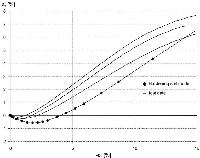
Figure 10.9 Results of drained triaxial tests on dense Hostun sand, volumetric strain versus axial strain
