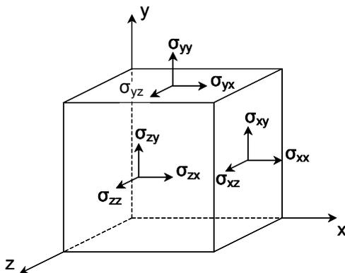
Figure 2.1 General three-dimensional coordinate system and sign convention for stresses
