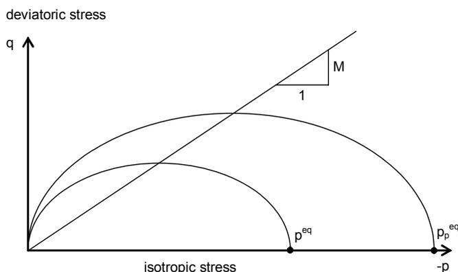
Figure 7.3 Diagram of  $p^{eq}$ -ellipse in a  $p$ - $q$ -plane
