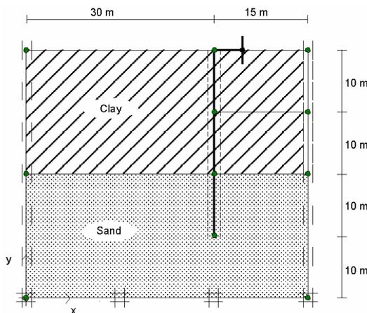
Figure 10.27 Geometry model of submerged excavation
