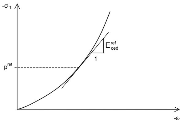
Figure 5.4 Definition of  $E_{oed}^{ref}$  in oedometer test results
