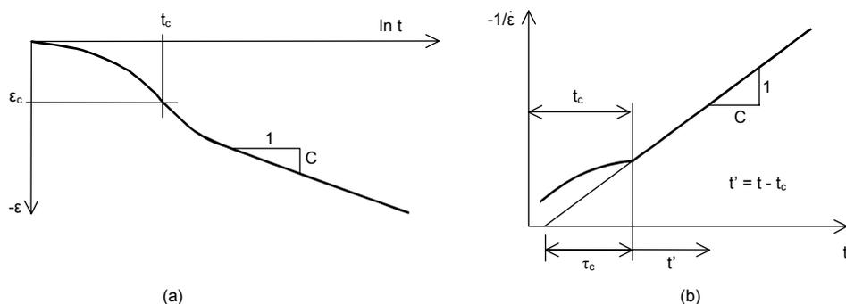
Figure 7.1 Consolidation and creep behaviour in standard oedometer test
