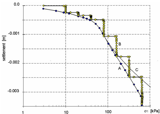
Figure 10.23 Load-settlement curve of oedometer test with Soft Soil Creep model. A) Transient loading with doubling of loading within one day. B) Instantaneous loading with doubling of load at the beginning of a new day. C) As 'A' using Updated Mesh calculation
