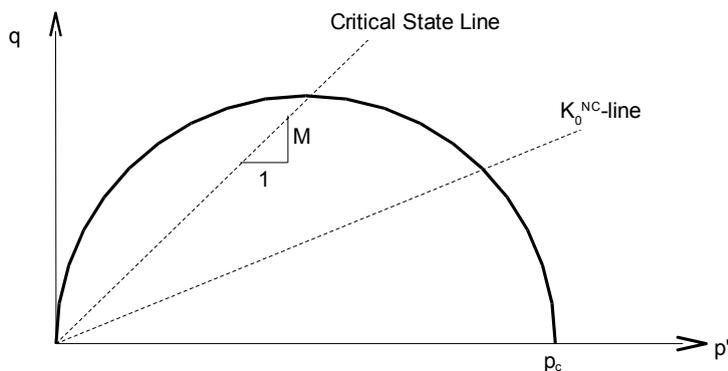
Figure 9.1 Yield surface of the Modified Cam-Clay model in  $p'$ - $q$ -plane
