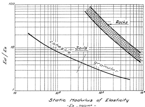
Figure 6.6 Relation between dynamic ( $E_d = E_0$ ) and static soil stiffness ( $E_s \approx E_{ur}$ ) after Alpan [46].
