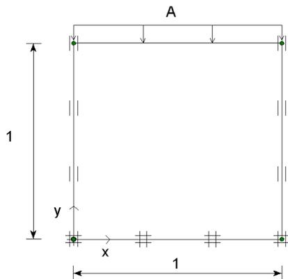
Figure 10.10 Simplified configuration of an oedometer test
