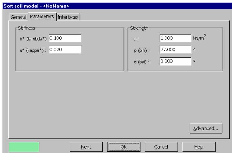
Figure 8.4 Parameters tab sheet for the Soft Soil model
