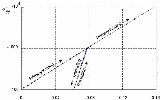
Figure 10.26 Results of isotropic compression test
