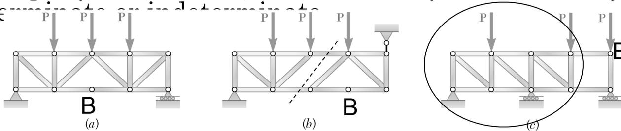
(a)  $2j = 20$ ,  $m = 16$ ,  $r = 3$ . *Non-simple with  $2j > m + 3$* , and thus the truss is **partially constrained**. The truss is **not** internally rigid. A vertical load at point B cannot be balanced.
