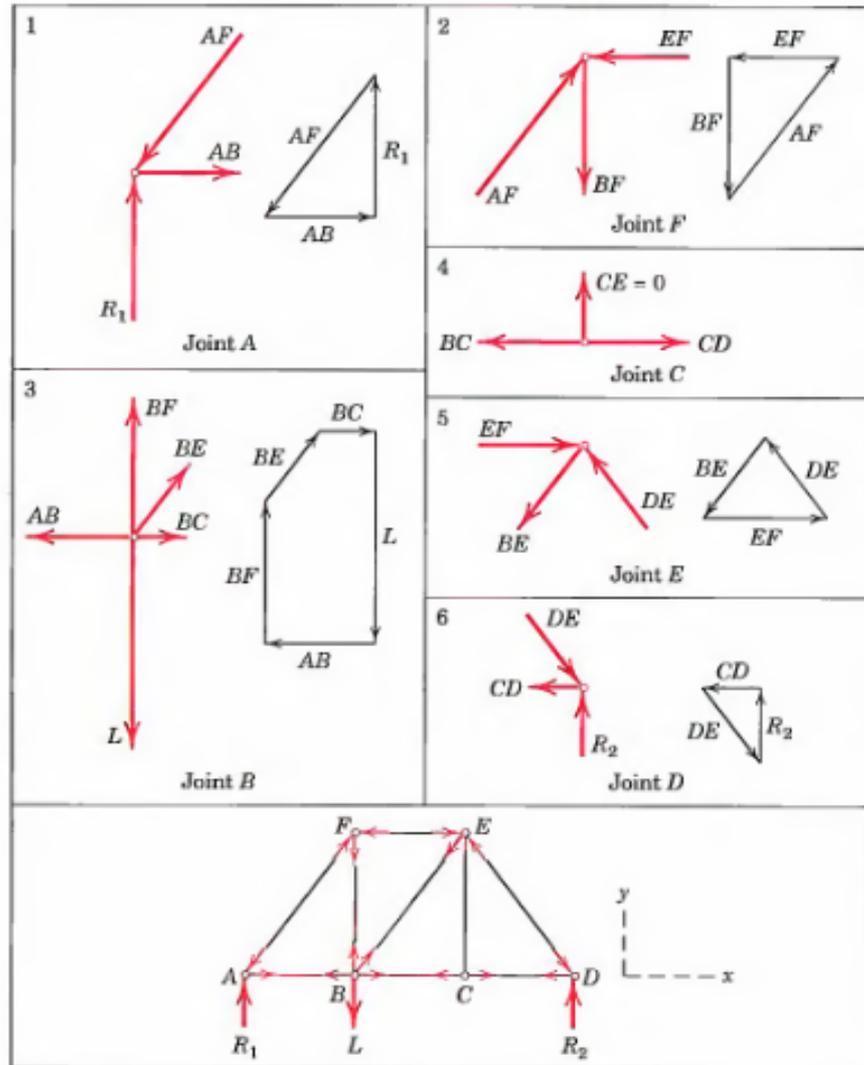
Note the direction of the forces in the members acting on the joints
