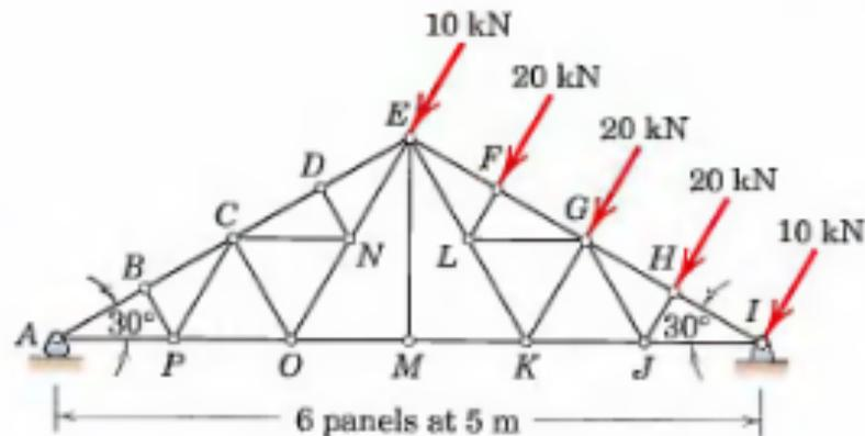
$$EF = 75.1 \text{ kN (C)}, KL = 40 \text{ kN (T)}, GL = 20 \text{ kN (T)}$$
