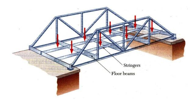
Members of a truss are slender and not capable of supporting large lateral loads. Loads must be applied at the joints.
