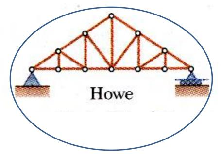
• A simple truss is constructed by successively adding two members and one connection to the basic triangular truss.
