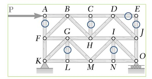
• Joint E is connected to two members which are not in a straight line.
