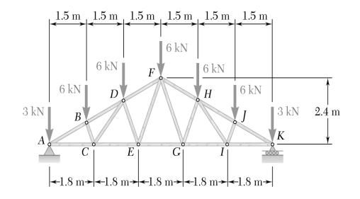
• Use method of section to determine the force in members IK, HK, FI, EG of the truss shown in the figure.
