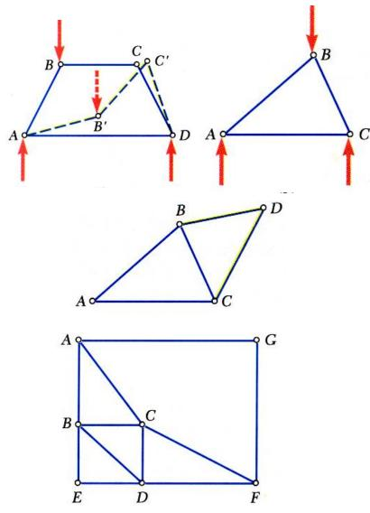
• A rigid truss will not collapse under the application of a load.
