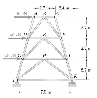
• The truss supports a ramp (shown with a dashed line) which extends from a fixed approach level near joint F to a fixed exit level near J. The loads shown represent the weight of the ramp. Determine the forces in members BH and CD.
