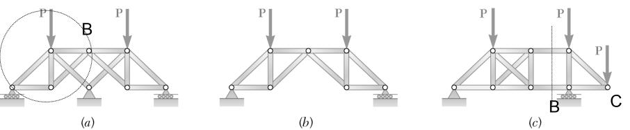
a)j = 8, m = 12, r = 4, 2j = m + r. But note that for the left truss, moment balance about B is not obeyed. So the truss is **Improperly constrained**
