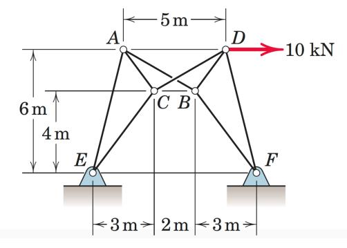
• Determine the forces in bars 1. 2. and 3 of the plane truss supported and loaded as shown in the figure
