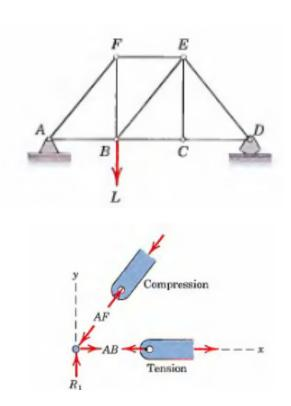
Note the direction of the forces in the members acting on the joints
