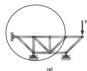
determinate or indeterminate (a)  $\mathbf{j} = \mathbf{8}$ ,  $\mathbf{m} = \mathbf{12}$ ,  $\mathbf{r} = \mathbf{4}$ ,  $\mathbf{2j} = \mathbf{m} + \mathbf{r}$ . Seemingly the truss is completely constrained. The circled portion is *simple* and adequately constrained with 3 reactions. The remaining portion can take care of any loading. Also not possible to deform the parallelogram. Completely constrained.
