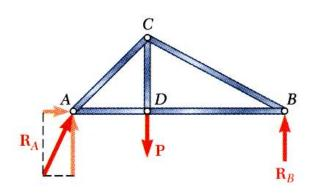
• Use conditions for equilibrium for the entire truss to solve for the reactions  $R_A$ and  $R_B$ .
