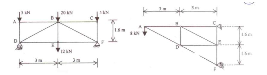
• For the given loading , determine the zero force member in the truss shown
