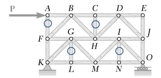
• Joint C is connected to three members out of which members CB and CD are in straight lines.
