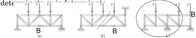
(a) 2j = 20, m = 16, r = 3. *Non-simple with* **2j > m + 3**, and thus the truss is *partially constrained*. The truss is *not* internally rigid. A vertical load at point B cannot be balanced.
