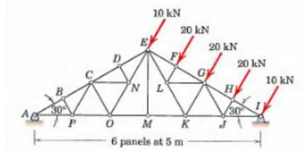
EF = 75.1 kN (C), KL = 40 kN (T), GL = 20 kN (T)
