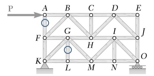
• Joint A is connected to two members and subjected to an external load P oriented along member AB.
