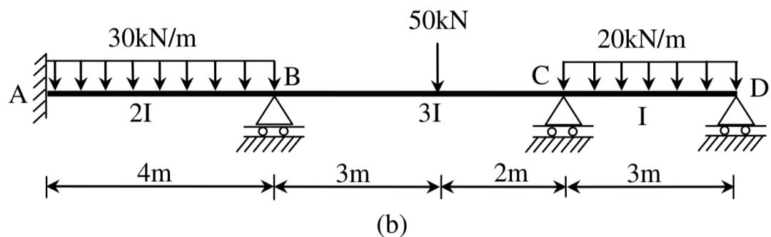
2. Analyse the frames shown in the figure using the moment distribution method. Use  $EI$  to be same for all the members.
