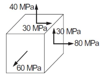
The stress matrix (tensor) corresponding to the state of stress shown is
