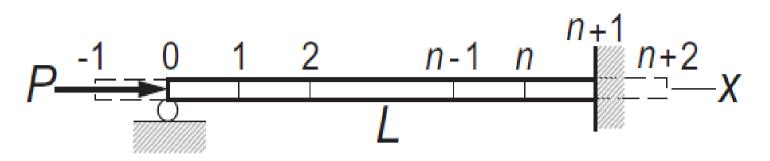
The propped cantilever beam carries a compressive axial load P. The lateral displacement u(x) of the beam can be shown to satisfy the differential equation
