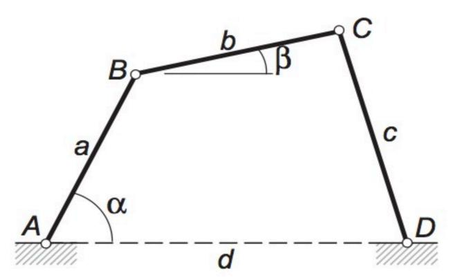
The linkage shown has the dimensions a=100 mm, b=120 mm, c=150 mm, and d=180 mm. It can be shown by geometry that the relationship between the angles  $\alpha$  and  $\beta$  is
