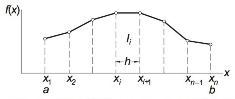
the region (a, b) divided into n - 1 panels, each of width h. we obtain for the approximate area of a typical (ith) panel
