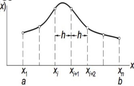
Simpson's 1/3 rule can be obtained from Newton–Cotes formulas with n = 3; that is, by passing a parabolic interpolant through three adjacent nodes, as shown in Fig. 6.4. The area under the parabola, which represents an approximation of  $\int_a^b f(x) dx$ , is
