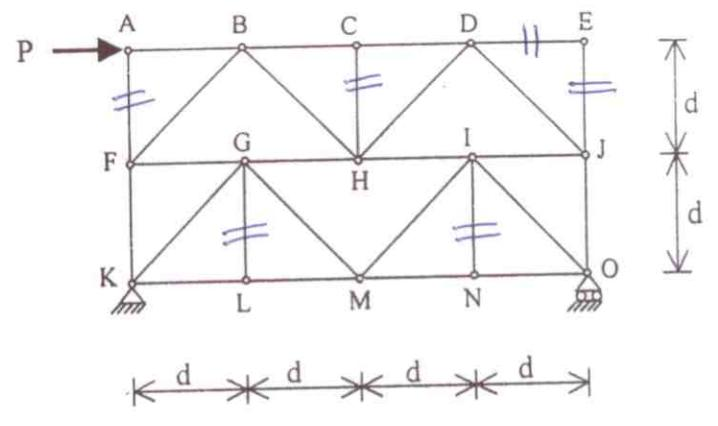
P.33. Determine the forces in members CD and DE of the truss shown
