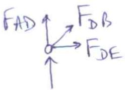
$F_{DE} + F_{DB} \left( \frac{3}{3.4} \right) = 0 \rightarrow F_{DE} = 30 (T) = F_{EF}$
