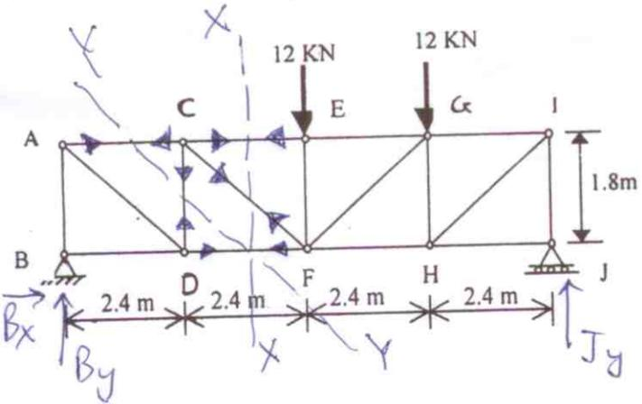
P.34. Determine the forces in members DF and DE of the truss shown.
