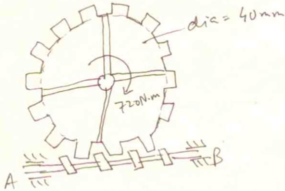
should be applied to wheel to keep it rolling @ uniform speed. (3)
