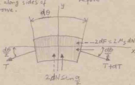
$$\sum F_y: 2dN \sin \frac{\alpha}{2} - 2T \sin \frac{d\theta}{2} - dT \sin \frac{d\theta}{2} = 0 \Rightarrow dN \sin \frac{\alpha}{2} - T d\theta = 0$$
