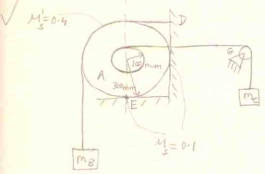
Given:  $W_C = 500N, W_A = 100N, G$  is frictionless pulley
