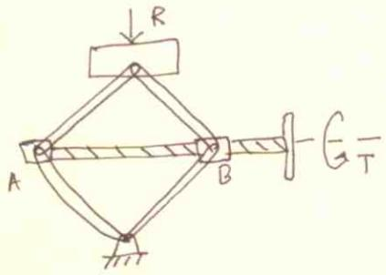
Given: scissors jack lifting car. 'A' is merely a bearing, 'B' is a threaded collar (nut). Single threaded screw with pitch  $p = 3 \text{ mm}$ , mean dia =  $2r = 20 \text{ mm}$ ,  $\mu_s = 0.3$ . Find  $T$  for  $\theta = 45^\circ$  and  $60^\circ$ .
