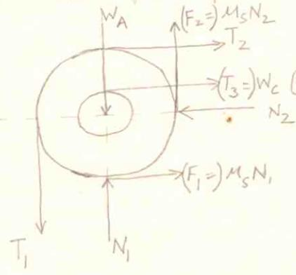
Note: we must take  $T_1 > T_2$  if we want to use the form  $(T_1/T_2) = e^{\mu \theta}$
