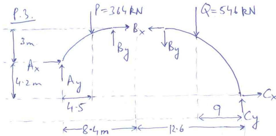
$$\text{Left FBD: } \sum M_A = 0 \Rightarrow (364)(4.5) + B_x(3) - B_y(8.4) = 0 \quad \left. \begin{array}{l} B_x = -630 N \\ B_y = -30 N \end{array} \right\} \blacktriangleleft$$
