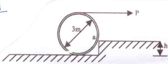
1. What is the height  $h$  of the step shown in the figure so that the force  $P$  will roll the 25 kg cylinder over the step at the same time that there is impending slippage at  $a$ ? Take coefficient of static friction = 0.3.
