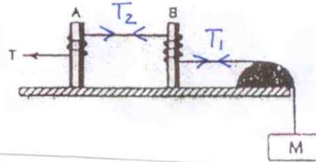
$Mg > T_1 > T_2 > T$  for impending downward motion of M.
