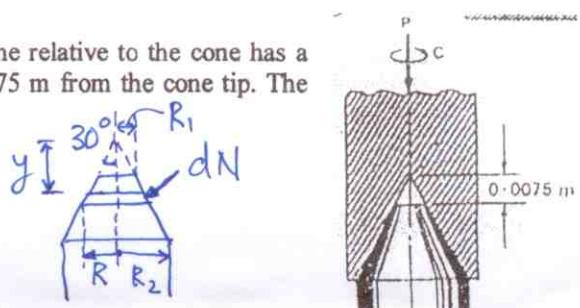
$$\sum F_y : P = \left( \int_A p dA \right) \sin 30^\circ = p \sin 30^\circ * A \quad (\because p \text{ is uniform})$$
