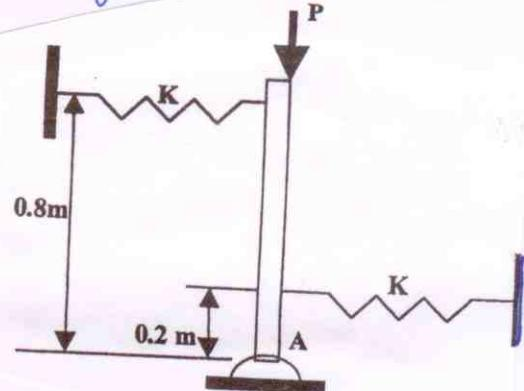
$$\begin{aligned} \sum M_A = I_A \ddot{\theta} &\rightarrow mg\left(\frac{l}{2}\theta\right) + P(l\theta) - K(0.8\theta)0.8 - K(0.2\theta)0.2 = \frac{ml^2}{3}\ddot{\theta} \\ &\rightarrow \frac{60}{9.81} \frac{(l)^2}{3} \ddot{\theta} + [K(0.8^2 + 0.2^2) - \frac{mg}{2}] \theta = 0 \\ \omega_n &= \sqrt{\frac{[0.68K - \frac{mg}{2}] 9.81}{20}} \end{aligned}$$
