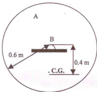
6. A disc weighs 445 N and has a radius of gyration of 0.45 m about its axis of symmetry. Note that the centre of gravity does not coincide with the geometric centre. Determine the natural frequency of oscillation. If at the instant that the centre of gravity is directly below B, the disc is rotating at a speed of 0.01 rad/sec counter-clockwise, determine the oscillation amplitude.
