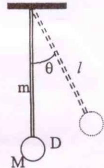
$$I_0 \ddot{\theta} = \sum M_0 \Rightarrow \left[ \frac{ml^2}{3} + \frac{2}{5} M \frac{D^2}{4} + M \left( l + \frac{D}{2} \right)^2 \right] \ddot{\theta} = -mg \frac{l}{2} \theta - Mg \left( l + \frac{D}{2} \right) \theta \rightarrow \text{EOM}$$
