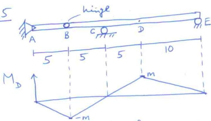
Moving point load of 4000 N, moving uniform load of 300 N/m applied. Self wt is 200 N/m.
