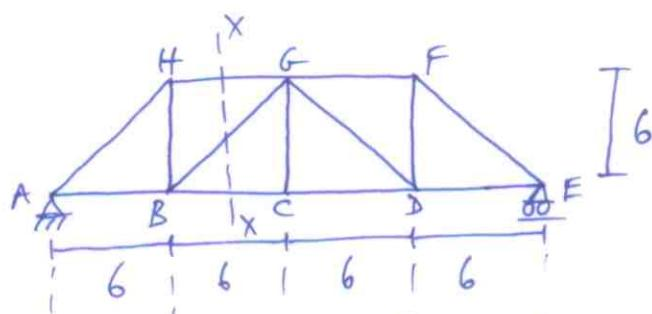
GC = zero force member unless point load applied at C.
