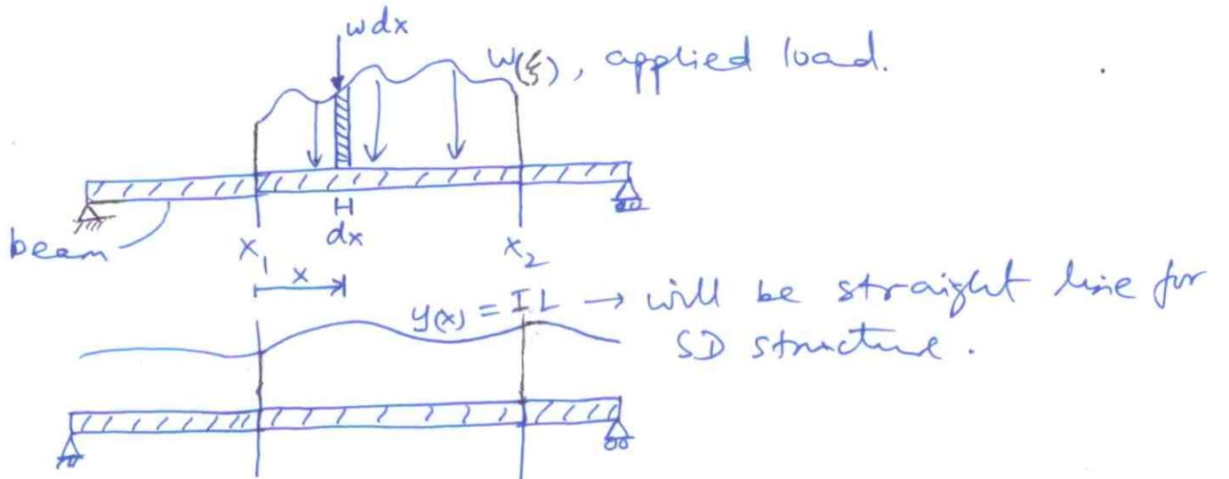
Represent  $w(\xi)$  as series of point loads  $w dx$  as shown. Value of influence function due to  $w dx$  applied at  $x$  is  $(w(\xi) dx) y(x)$ , ie  $y$  scaled by actual applied load  $w dx$ . Thus value of influence function due to total  $w(\xi)$ , applied over  $[x_1, x_2]$ , is sum of values due to individual  $w dx$ 's, ie,
