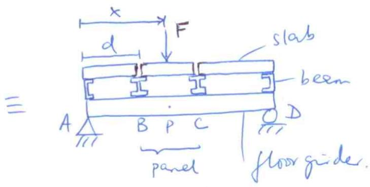
⇒ SF constant over a panel of the beam.  $R_{Ax} \rightarrow R_{Ay}$
