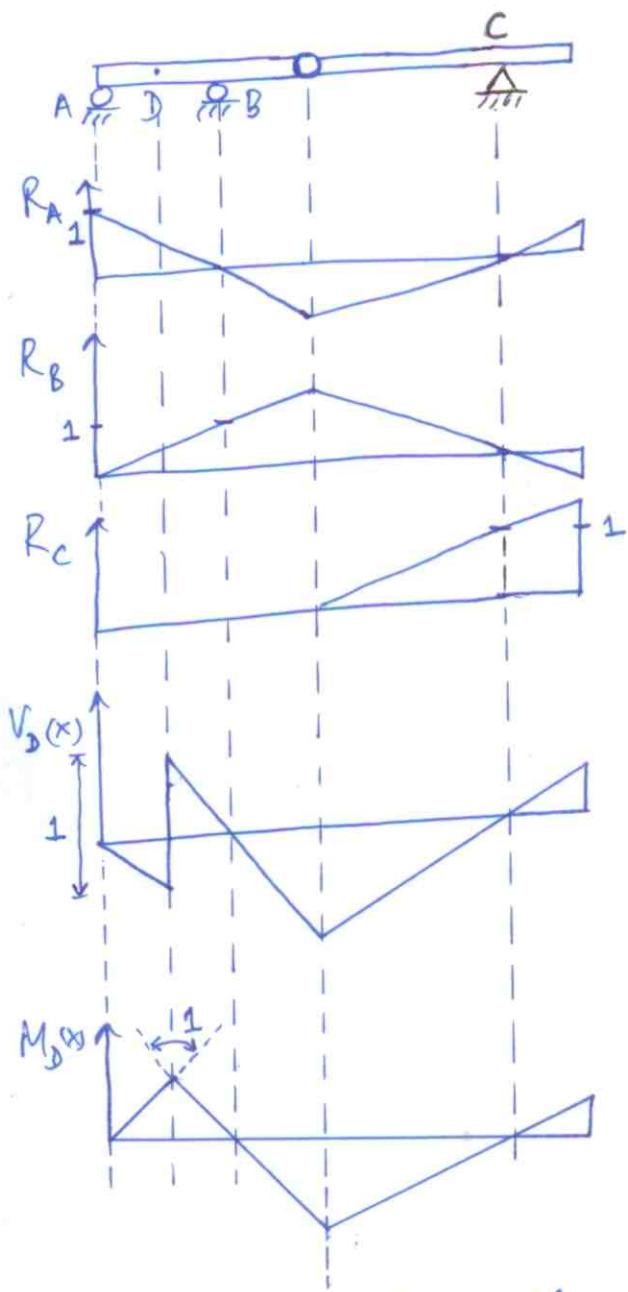
For  $R_A, R_B, R_C$ , release the support A, B, C, respectively and plot deflected shape maintaining constraint at remaining supports.
