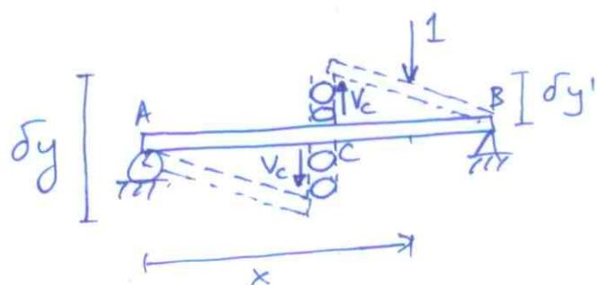
$$VW=0 = V_c \delta y - 1 \delta y' \\ = 1, \text{ chosen for convenience, w/o loss of generality} \\ \therefore V_c = \delta y'$$
