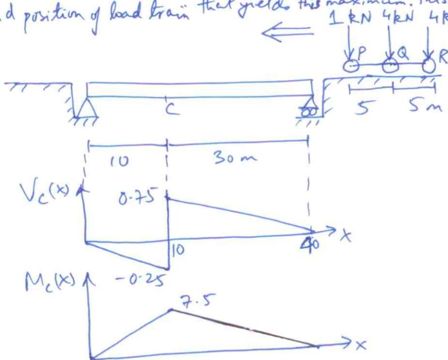
Due to piecewise-linear nature of IL, it is obvious that max will occur when one of the loads is at the point (station) where max value of IL occurs, i.e., at point C.
