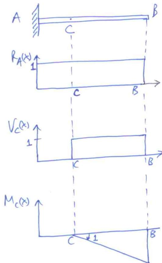
For  $R_A$ , release vertical reaction at A, keeping all other constraints at A intact (ie no rotation, horizontal translation).
