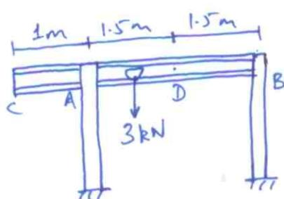
Hoist supported on beam CB weighing 24 kg/m. It carries 3 kN load. Assume A is pin, B is roller. Find max reactions at A, B and moment at D.
