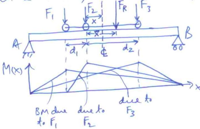
So we assume, or demand, that max BM occurs under a chosen load. Then we find the position ' $x$ ' of that load wrt  $\ell$  (i.e. in effect the position of the train) so that max BM occurs under that load. Then find the max BM for that position (i.e. BM under the chosen load). Then choose another load under which max BM should occur & repeat process. Finally choose absolute-max BM and corresponding load train position.
