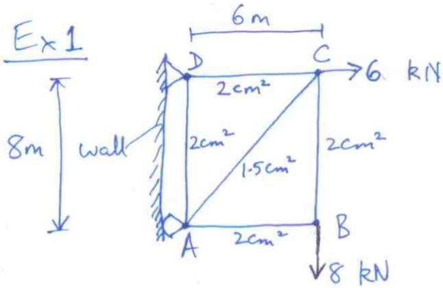
Find vertical displ of joint C due to applied loads as shown and temp change
