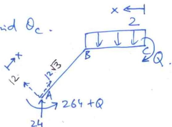
$$M = -(264+Q) + 12x, \quad \frac{\partial M}{\partial Q} = -1, \quad \text{in } AB.$$
