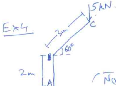
Ex 4 Find rotation at C. Take E = 200 GPa, I = 15E6 mm<sup>4</sup>. Consider effects of shear & axial deformation.
