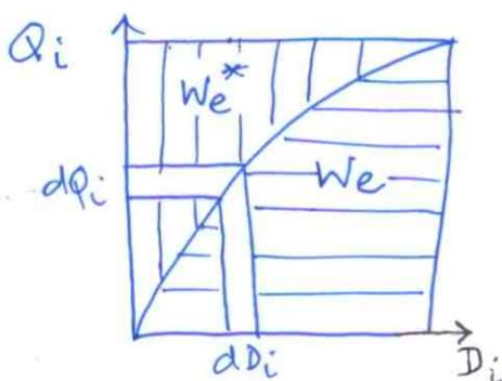
$$W_e = \int_0^{D_i} Q_i dD_i = \text{work done by real } Q_i \text{ undergoing real } D_i$$
