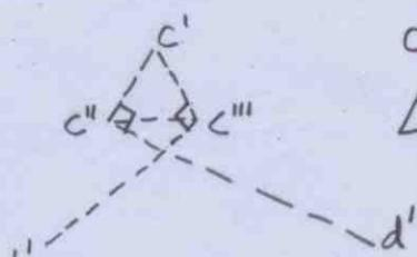
$$\begin{aligned} cc''' &= \Delta_b, cc'' = \Delta_c \\ \angle c'c''c''' &= \angle c'c''c''' \\ &= \frac{\pi}{2} - \angle c'''c''d' \\ &= \frac{\pi}{2} - \tan^{-1} \frac{10}{20} \end{aligned}$$
