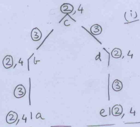
(i) Joints a, b, c, d, e shown with no. of unknowns shown, without encircling, against each joint. Note that only force unknowns (i.e., axial, shear or  $x, y$  forces) are being accounted for, since BM unknowns are assumed known from S-D eqns in terms of the displacements. Each joint has two force equilibrium equations (shown as ②). Note that moment equilibrium at a jt. (e.g.  $M_{cd} + M_{cl} = 0$ ) is already accounted in S-D method, so not accounted in this discussion.
