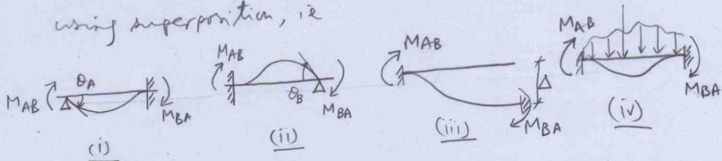
$$(i) + (ii) \quad EIw^{IV} = 0 \\ w = c_1 \frac{x^3}{6} + c_2 \frac{x^2}{2} + c_3 x + c_4$$
