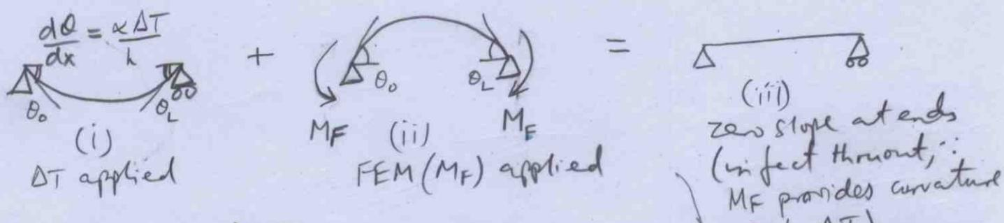
Note: from here itself you see that "MF provides constant curvature w'' wrt x, it should provide curvature equal in magnitude to  $d\theta/dx$
