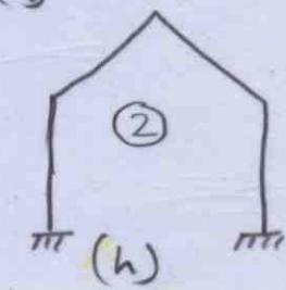
Degree of sidesway (instability) is noted against each frame. Frame (a) is statically unstable when converted to pin-joints (apply horizontal load and see it). All other frames are kinematically unstable (ie form mechanism) when converted to pin-joints. The number of links to be introduced to make them stable is shown below:
