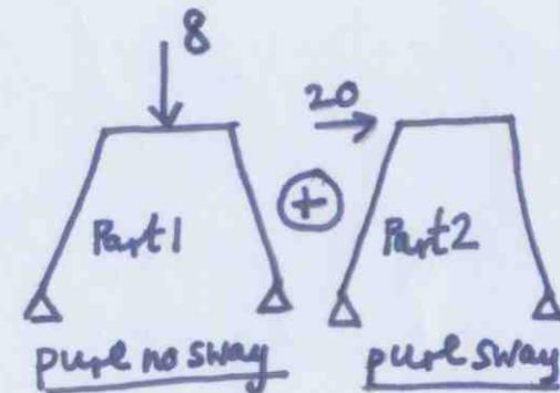
$$\text{Fem\_ba} = 3EI\Delta/\text{Lab}^2 = 100; \text{Fem\_bc} = 6EI\Delta/\text{Lbc}^2; \\ \Delta = 2\Delta_1 \sin \alpha; \sin \alpha = 3/5; \\ \text{Fem\_bc} = 2^2 * 3/5 * \text{Fem\_ba}; \\ \text{Va} = -(M_{ab} + M_{ba})/\text{Lab}; \text{Vd} = -(M_{cd} + M_{dc})/\text{Lcd}; \\ Fx * 5 * \cot \alpha = (\text{Va} + \text{Vd}) * (10 + 5 / \sin \alpha);$$
