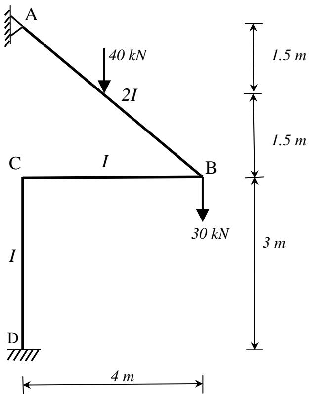
$$(1) EI \begin{bmatrix} \frac{4.4}{6} + \frac{4.1}{3} & \frac{2.1}{3} \\ \frac{2.1}{3} & \left(\frac{4.1+4.1+4.1}{3}\right) \end{bmatrix} \begin{Bmatrix} \theta_B \\ \theta_D \end{Bmatrix} = \begin{Bmatrix} -\frac{60.6}{8} + 10.2 \\ 0 \end{Bmatrix} \Rightarrow \text{No sway in given problem from equilibrium of jts B, D.}$$
