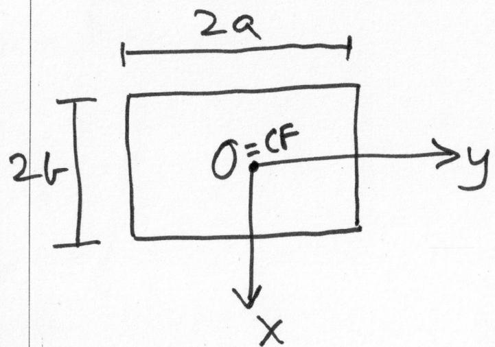
If load  $(w_x, w_y)$  applied at  $(x_0, y_0)$  find twisting moment  $M_2$  from ⑩ p. 28 with  $(x_{CF}, y_{CF}) = (0, 0)$ , and solve torsional shear stresses  $\tau_{xz}, \tau_{yz}$  due to  $M_2$  by FDM for torsion.
