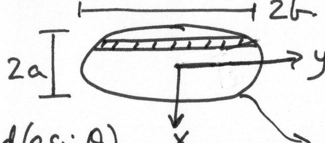
$$\begin{aligned} Q &= \int_A x dA = \int_A a \sin \theta \cdot 2b \cos \theta \cdot d(a \sin \theta) \\ &= \int_0^{\pi/2} 2a^2 b \cos^2 \theta \sin \theta \, d\theta = \frac{2}{3} a^2 b \cos^3 \theta \end{aligned}$$
