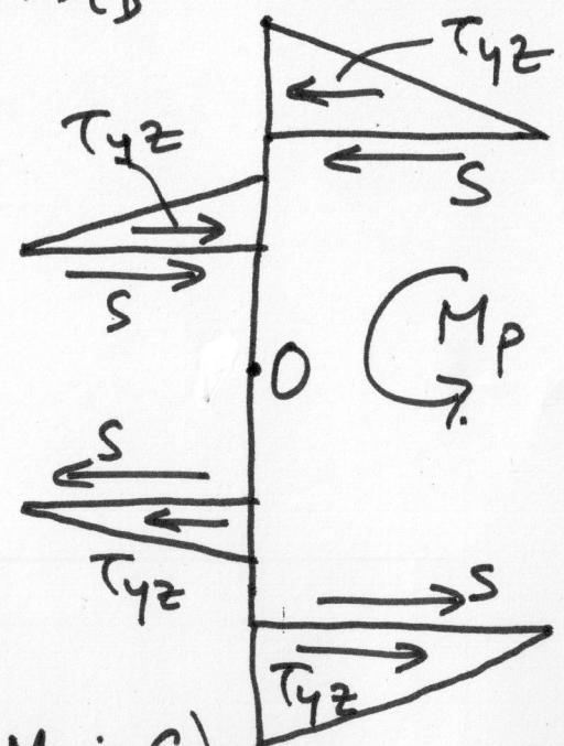
Shear center of section with ALL legs intersecting at a point, is the point of intersection.
