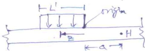
$$\Delta W_H = \frac{q \Delta z \beta}{2R} A_{\beta(z+a)} \quad \left( \text{using formula for point load from thin strip of distributed load} \right)$$
