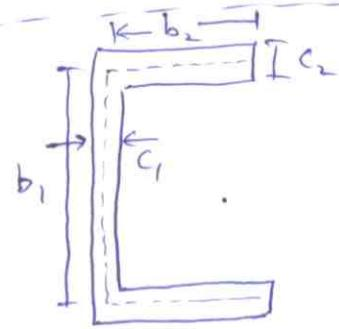
P.2  $\alpha \approx \frac{3M}{(b_1 c_1^3 + 2b_2 c_2^3)G}$
