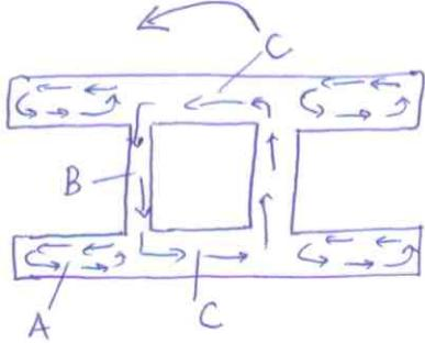
Since the four limbs are identical they contribute equal torsional moments. Let  $M_L$  = torsional moments in all 4 limbs.  $M_B$  = torsional moment in closed loop (box).
