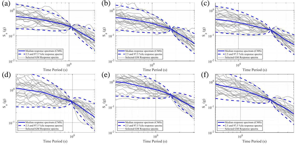
**Fig. 2.** Response spectra of selected ground motion suites along with conditional mean spectrum and 2.5–97.5%ile spectral ordinates for 2-, 4-, and 7-story buildings in (a, b, c) Zone-IV and in (d, e, f) Zone-V.
