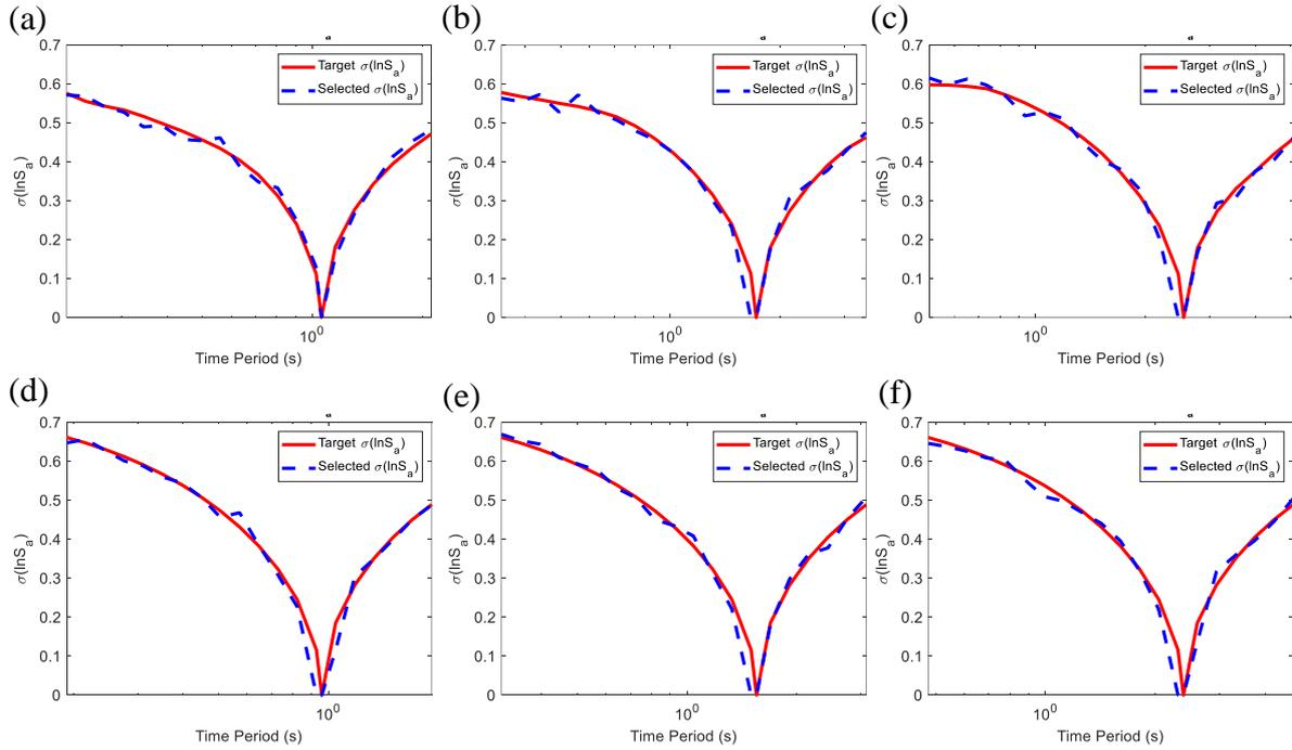
**Fig. 3.** Comparison of target and selected standard deviation in logarithm of spectral ordinates for 2-, 4-, and 7-story buildings in (a, b, c) Zone-IV and in (d, e, f) Zone-V.
