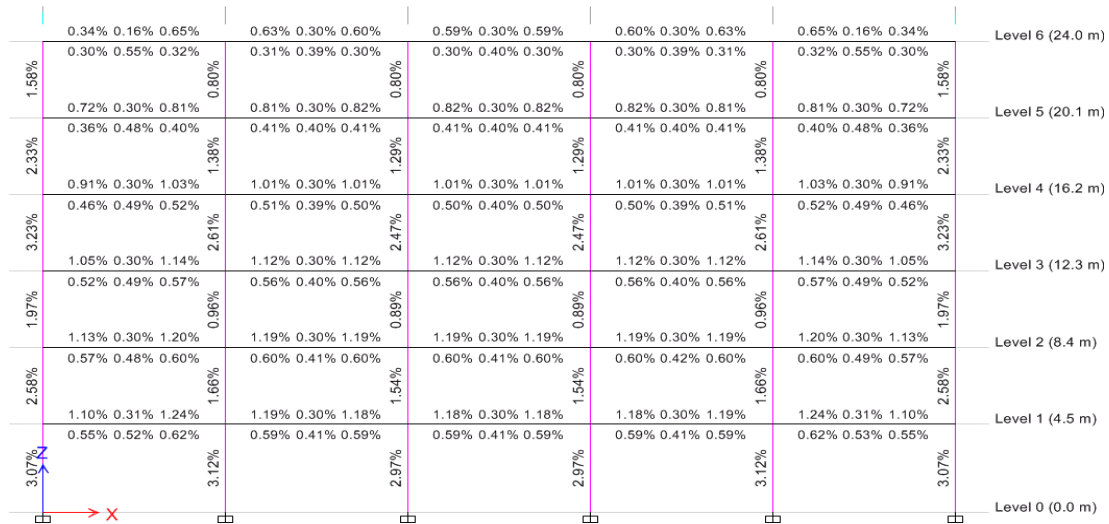
Fig. 21b. Required longitudinal reinforcement for building ID 2439
