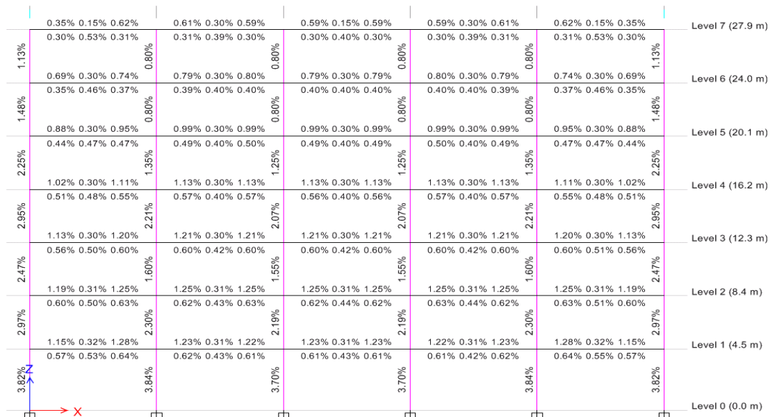
Fig. 22b. Required longitudinal reinforcement for building ID 2229
