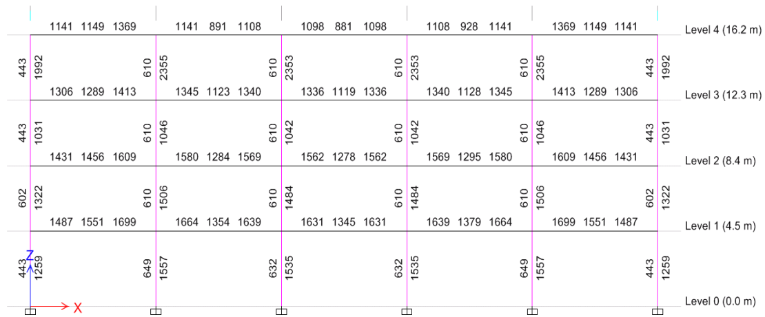
Fig. 19c. Required transverse reinforcement for building ID 2227
