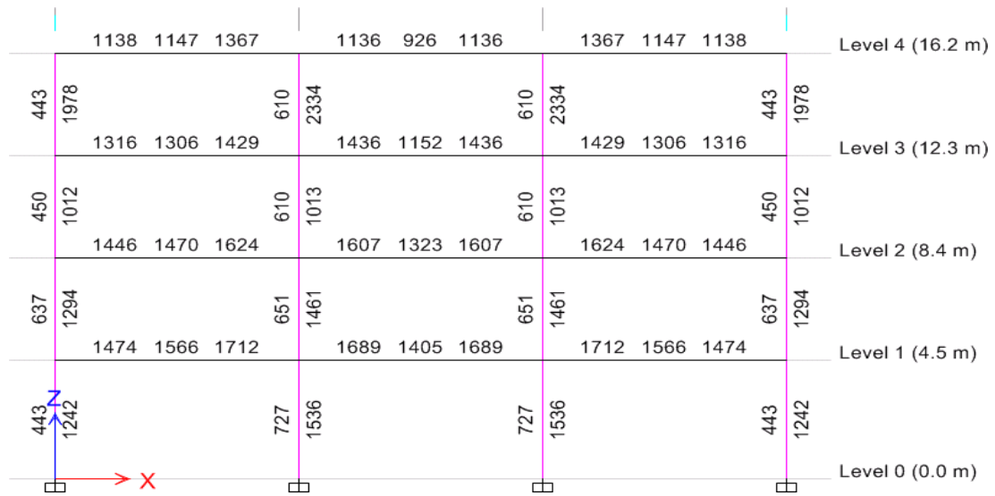
Fig. 10c. Required transverse reinforcement for building ID 2221
