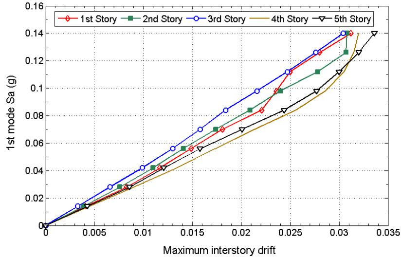
Figure 7. 95 percentile IDA curves for all the stories of the upgraded 5-story frame
