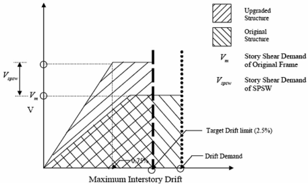
Figure 1. Schematic representation of the static energy based scheme used for upgrading
