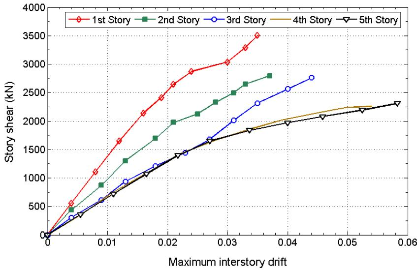
Figure 5. 95 percentile story shear versus maximum inter-story drift for the original 5-story frame
