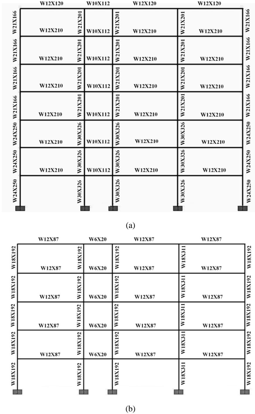
Figure 2. Elevations of the original: a) 7-story; and b) 5-story frames
