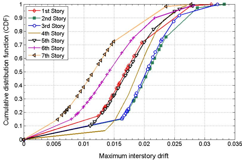
Figure 8. Cumulative distribution function of maximum inter-story drift at the selected hazard level for the upgraded 7-story frame
