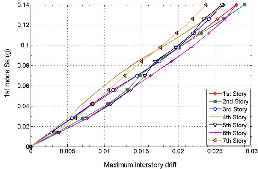
Figure 6. 95 percentile IDA curves for all the stories of the upgraded 7-story frame
