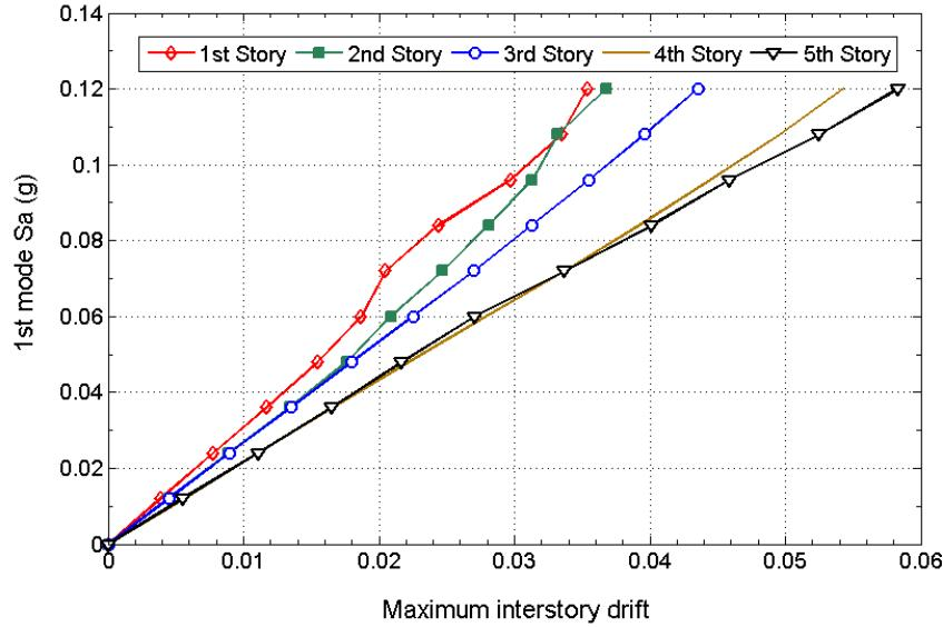
Figure 4. 95 percentile IDA curves for all the stories of the original 5-story frame
