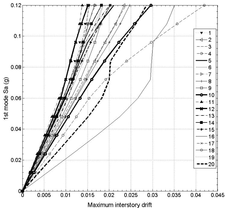
Figure 3. Multi-record IDA plot for the LMSR records for the 1st story of the original 5-story frame
