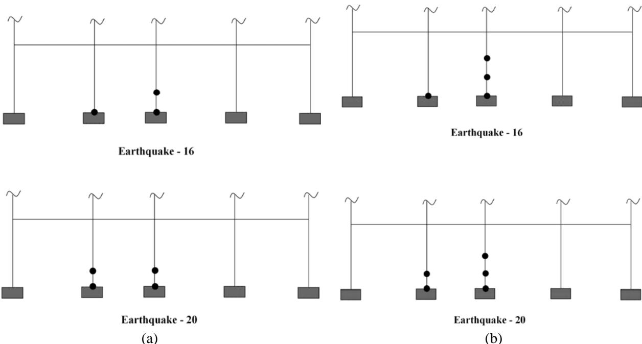
Figure 9. Plastic hinge formation in the boundary columns for the upgraded: a) 7-story; and b) 5-story frames
