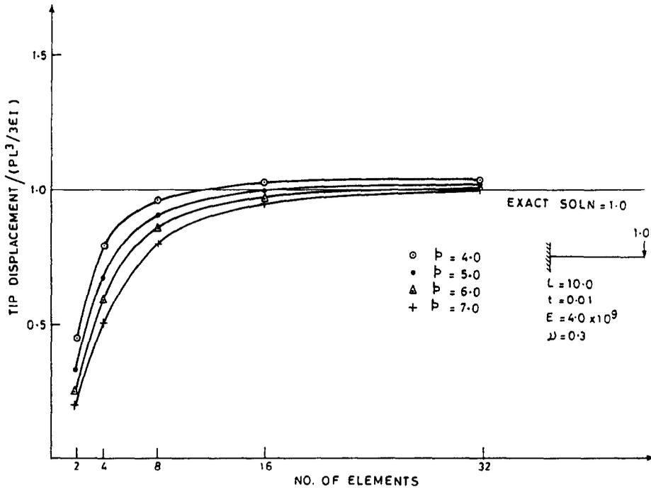
Fig. 3. Cantilever under tip load (see Table 1).
