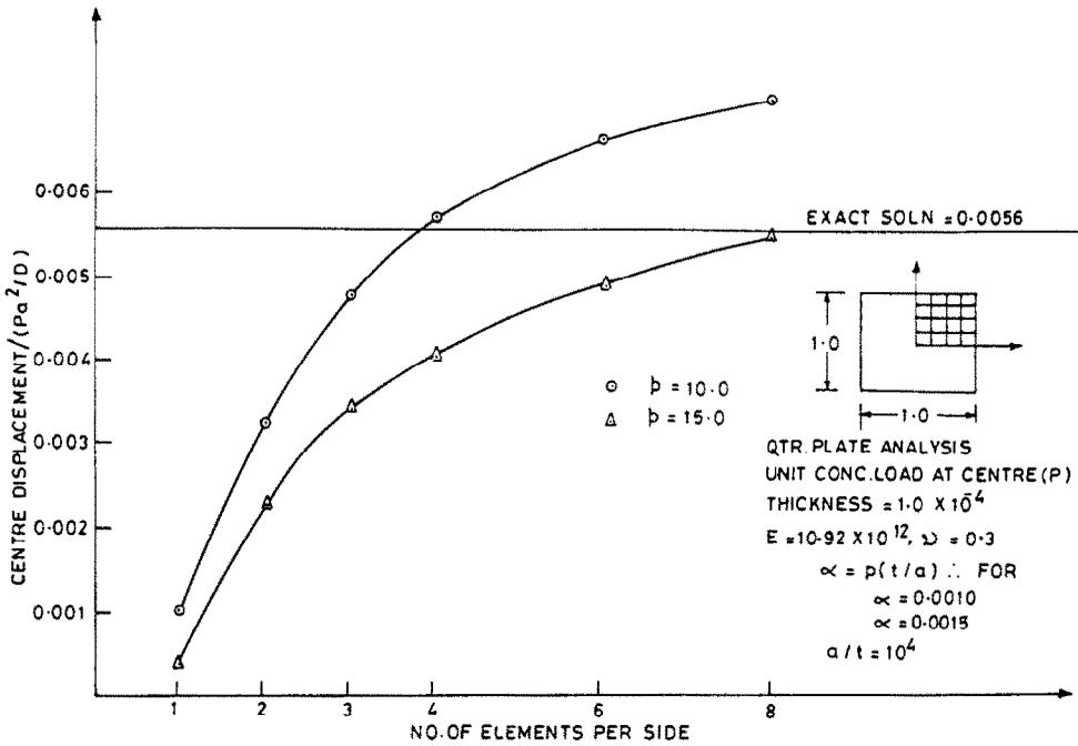
Fig. 11. Clamped plate under concentrated load at centre (see Table 9).
