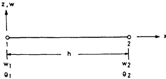
Fig. 1. 2-Noded linear element.
