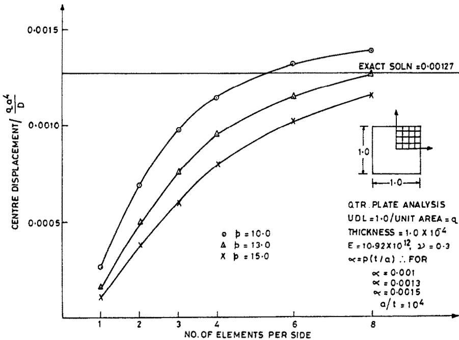
Fig. 12. Clamped plate under UDL (see Table 10).
