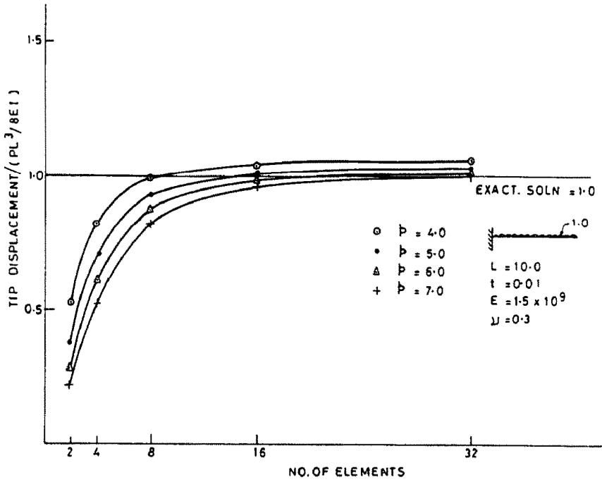
Fig. 4. Cantilever under UDL (see Table 2).
