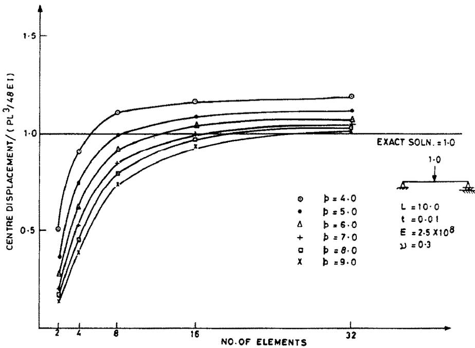
Fig. 5. Simply supported beam under concentrated load at centre (see Table 3).
