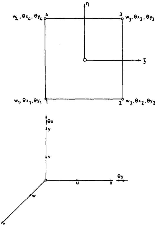
Fig. 2. 4-Noded quadrilateral element.
