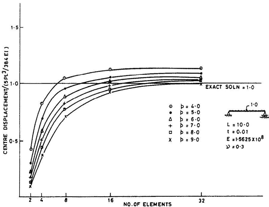
Fig. 6. Simply supported beam under UDL (see Table 4).
