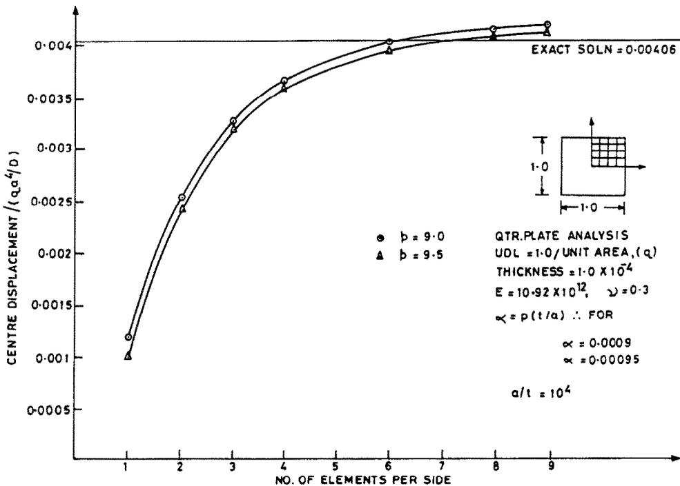
Fig. 10. Simply supported plate under UDL (see Table 8).
