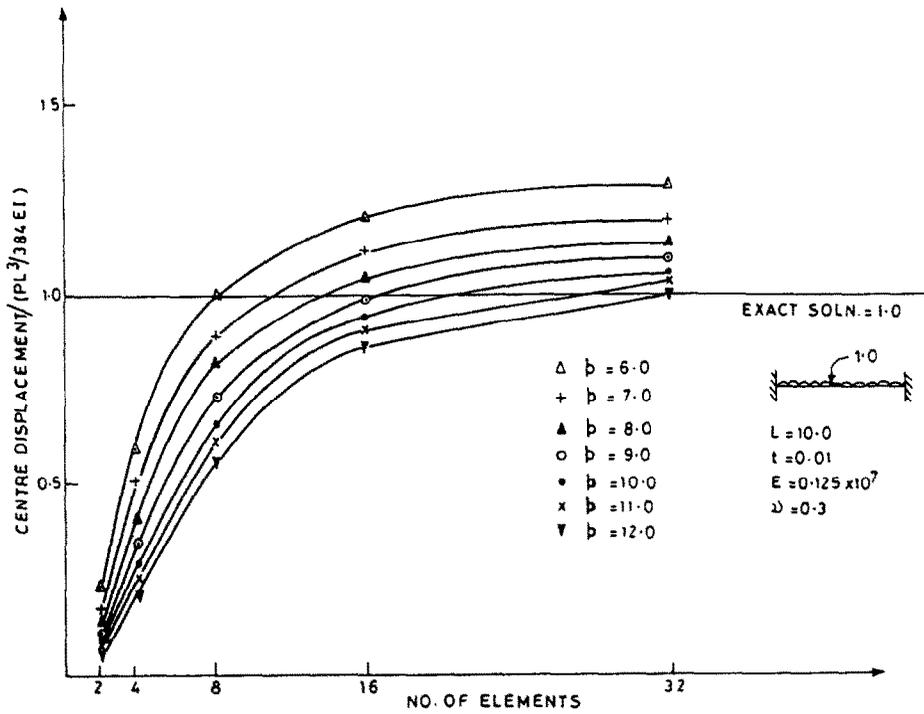
Fig. 8. Clamped beam under UDL (see Table 6).
