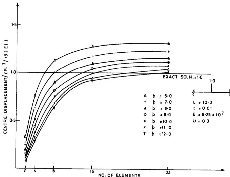
Fig. 7. Clamped beam under concentrated load at centre (see Table 5).
