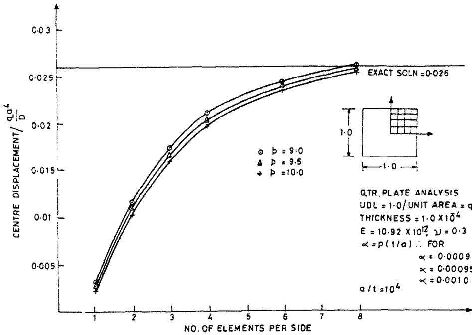
Fig. 13. Corner just supported plate under UDL (see Table 11).
