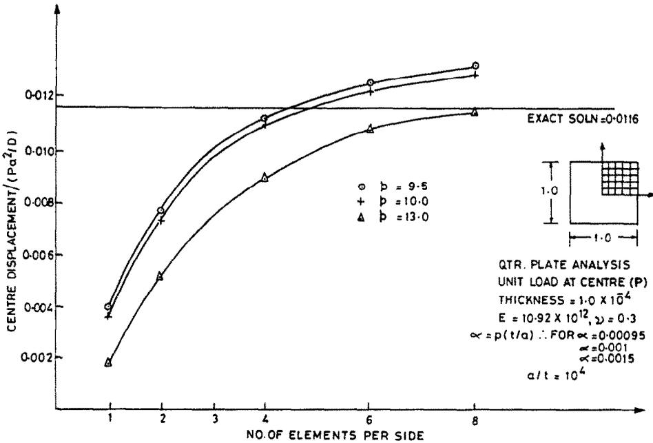
Fig. 9. Simply supported plate under concentrated load at centre (see Table 7).
