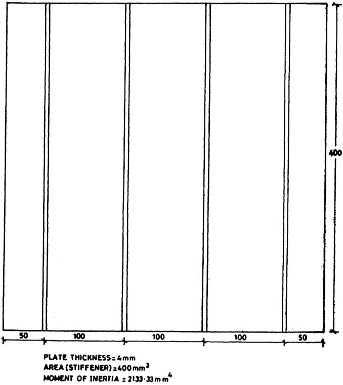
**Figure 1.** Plate configuration and material properties of the square plate with four stiffeners.
