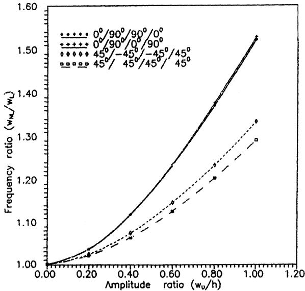
**Figure 5.** Variation of frequency ratio ( $w_{NL}/w_L$ ) of a square cross-stiffened composite plate with amplitude ratio ( $w_0/h$ ) for five different ply orientations (Case 3).
