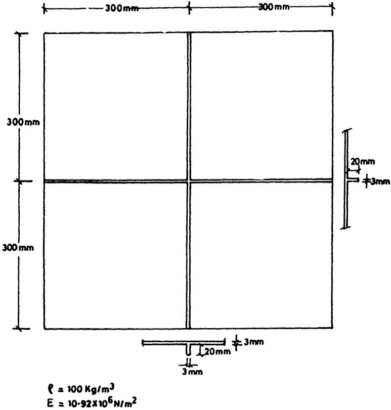
Figure 2. Plate and stiffener configuration of cross-stiffened square plate.
