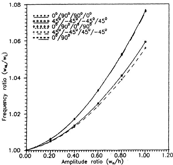
Figure 4. Variation of frequency ratio ( $w_{NL}/w_L$ ) of a square cross-stiffened composite plate with amplitude ratio ( $w_0/h$ ) for five different ply orientations (Case 2).
