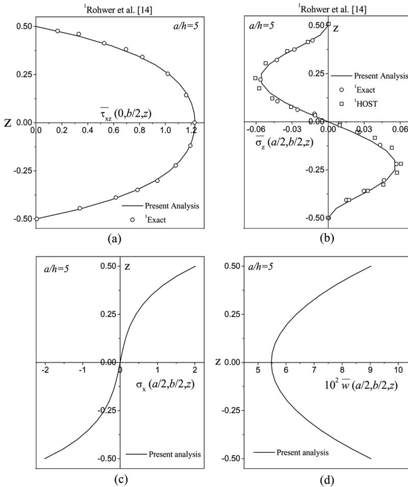
**Figure 4** Variation of normalized (a) transverse shear stress  $\bar{\tau}_{xz}$  (b) transverse normal stress  $\bar{\sigma}_z$  (c) inplane normal stress  $\bar{\sigma}_x$  (d) transverse displacement  $\bar{w}$  through thickness of a homogeneous orthotropic plate subjected to thermal load,  $\Delta T(x, y, h/2) = -\Delta T(x, y, -h/2) = T_0 \sin \frac{\pi x}{a} \sin \frac{\pi y}{b}$  (Case B).
