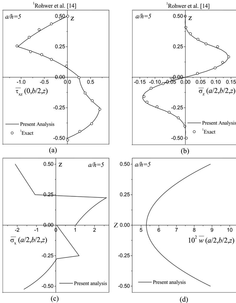
**Figure 8** Variation of normalized (a) transverse shear stress  $\bar{\tau}_{xz}$  (b) transverse normal stress  $\bar{\sigma}_z$  (c) inplane normal stress  $\bar{\sigma}_x$  (d) transverse displacement  $\bar{w}$  through thickness of a  $0^\circ/90^\circ/0^\circ/90^\circ$  unsymmetric composite subjected to thermal load,  $\Delta T(x, y, h/2) = -\Delta T(x, y, -h/2) = T_0 \sin \frac{\pi x}{a} \sin \frac{\pi y}{b}$  (Case B).
