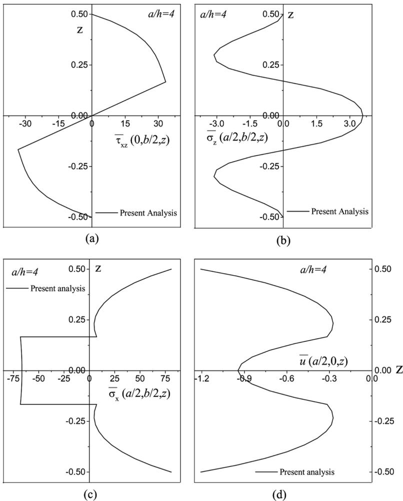
**Figure 5** Variation of normalized (a) transverse shear stress  $\overline{\tau_{xz}}$  (b) transverse normal stress  $\overline{\sigma_z}$  (c) inplane normal stress  $\overline{\sigma_x}$  (d) inplane displacement  $\overline{u}$  through thickness of a  $0^\circ/90^\circ/0^\circ$  symmetric composite plate subjected to thermal load,  $\Delta T(x, y, \pm h/2) = T_0 \sin \frac{\pi x}{a} \sin \frac{\pi y}{b}$  (Case A).
