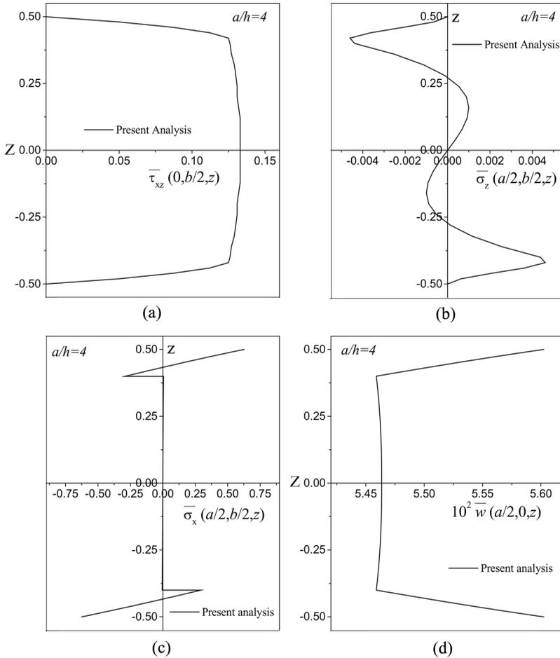
**Figure 10** Variation of normalized (a) transverse shear stress  $\tau_{xz}$  (b) transverse normal stress  $\sigma_z$  (c) inplane normal stress  $\sigma_x$  (d) transverse displacement  $w$  through thickness of a  $0^\circ/\text{core}/0^\circ$  symmetric sandwich subjected to thermal load,  $\Delta T(x, y, h/2) = -\Delta T(x, y, -h/2) = T_0 \sin \frac{\pi x}{a} \sin \frac{\pi y}{b}$  (Case B).
