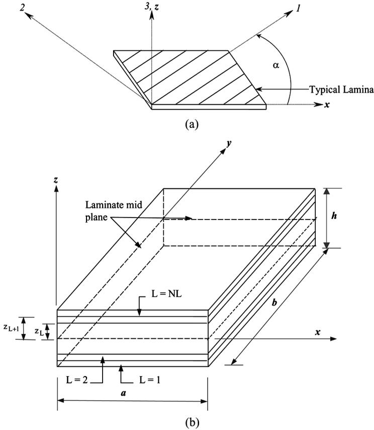
**Figure 1** Laminate geometry with positive set of lamina/laminate reference axes and fiber orientation.
