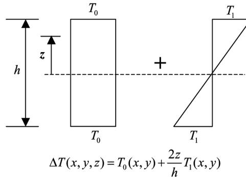
**Figure 2** Through thickness temperature distribution.
