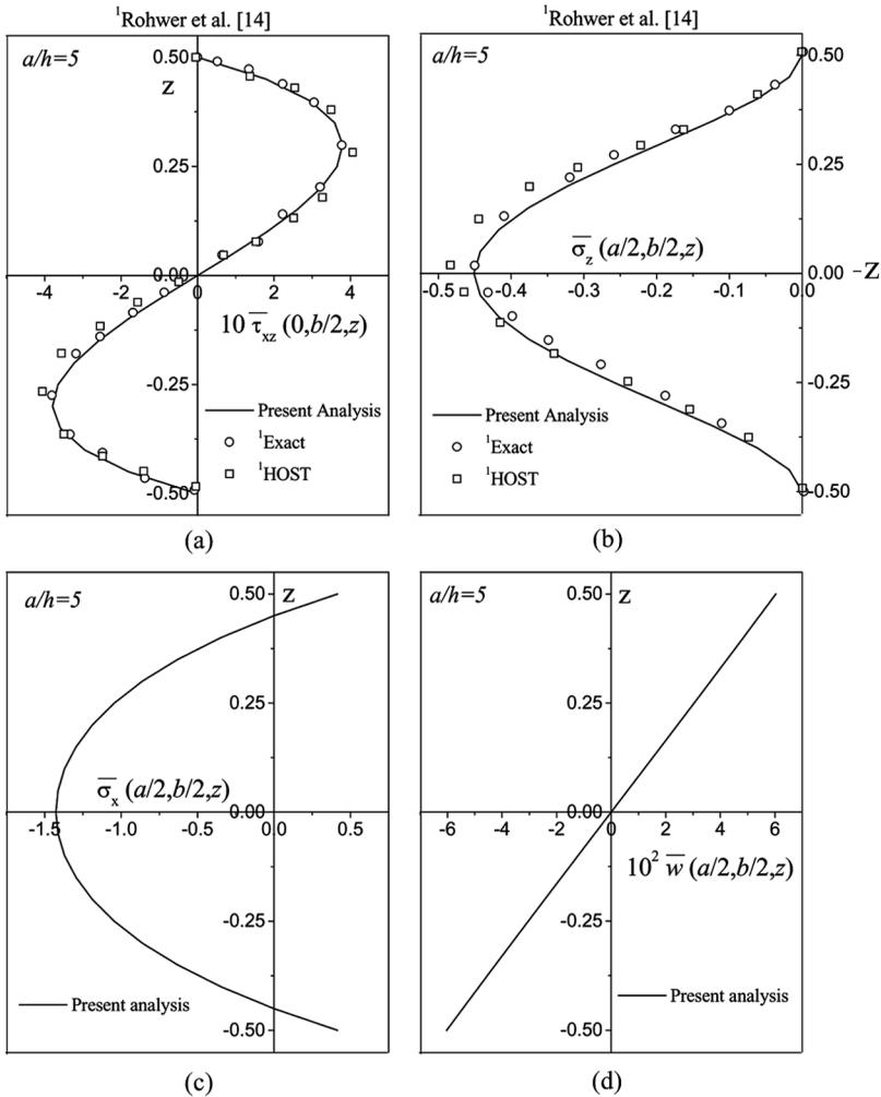
**Figure 3** Variation of normalized (a) transverse shear stress  $\bar{\tau}_{xz}$  (b) transverse normal stress  $\bar{\sigma}_z$  (c) inplane normal stress  $\bar{\sigma}_x$  (d) transverse displacement  $\bar{w}$  through thickness of a homogeneous orthotropic plate subjected to thermal load,  $\Delta T(x, y, \pm h/2) = T_0 \sin \frac{\pi x}{a} \sin \frac{\pi y}{b}$  (Case A).
