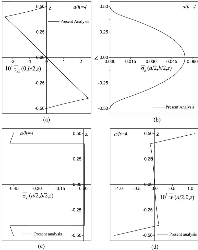
**Figure 9** Variation of normalized (a) transverse shear stress  $\bar{\tau}_{xz}$  (b) transverse normal stress  $\bar{\sigma}_z$  (c) inplane normal stress  $\bar{\sigma}_x$  (d) inplane displacement  $\bar{w}$  through thickness of a  $0^\circ/\text{core}/0^\circ$  symmetric sandwich plate subjected to thermal load,  $\Delta T(x, y, \pm h/2) = T_0 \sin \frac{\pi x}{a} \sin \frac{\pi y}{b}$  (Case A).
