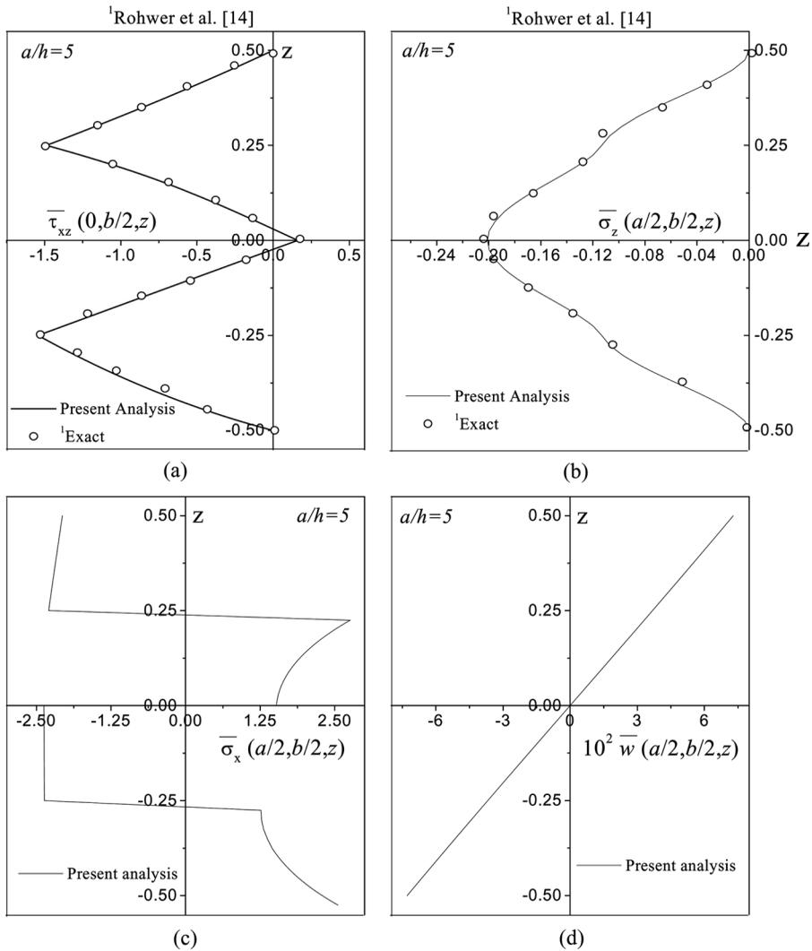
**Figure 7** Variation of normalized (a) transverse shear stress  $\overline{\tau}_{xz}$  (b) transverse normal stress  $\overline{\sigma}_z$  (c) inplane normal stress  $\overline{\sigma}_x$  (d) transverse displacement  $\overline{w}$  through thickness of a  $0^\circ/90^\circ/0^\circ/90^\circ$  unsymmetric composite plate subjected to thermal load,  $\Delta T(x, y, \pm h/2) = T_0 \sin \frac{\pi x}{a} \sin \frac{\pi y}{b}$  (Case A).
