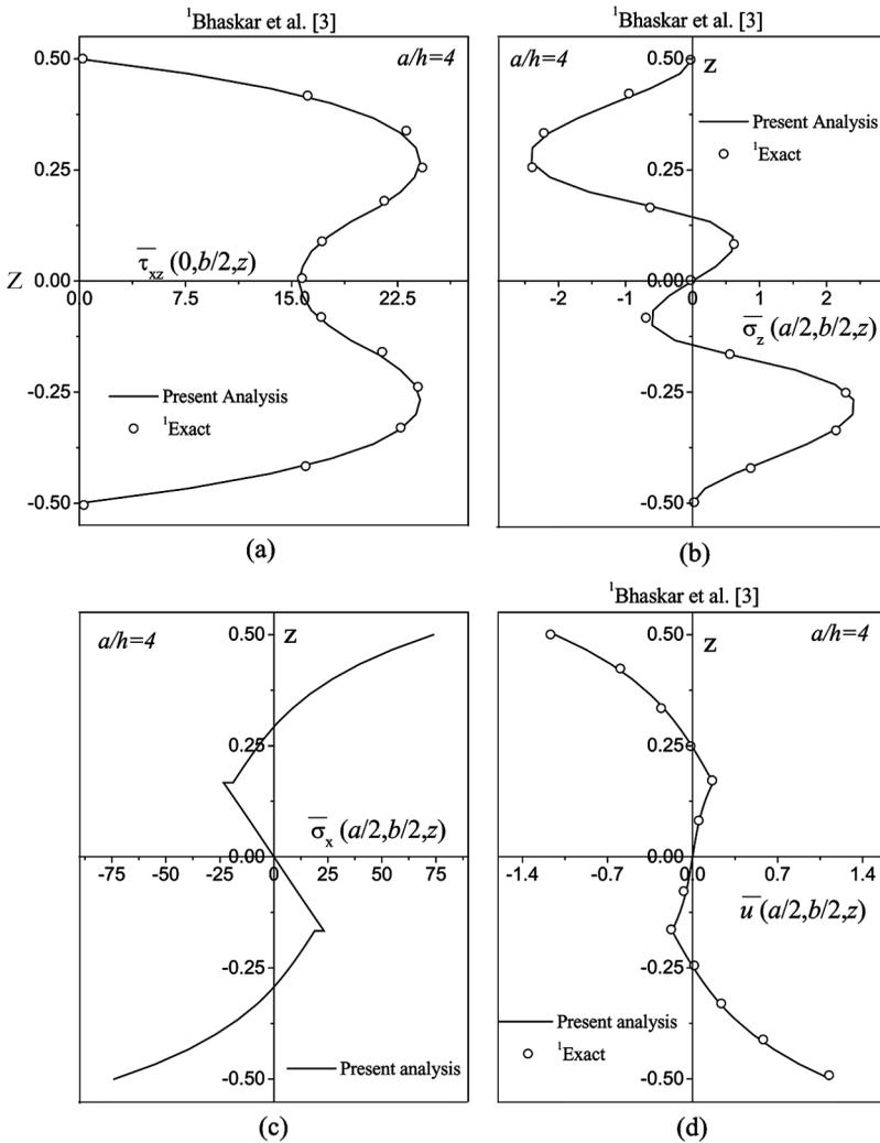
**Figure 6** Variation of normalized (a) transverse shear stress  $\bar{\tau}_{xz}$  (b) transverse normal stress  $\bar{\sigma}_z$  (c) inplane normal stress  $\bar{\sigma}_x$  (d) transverse displacement  $\bar{w}$  through thickness of a  $0^\circ/90^\circ/0^\circ$  symmetric composite subjected to thermal load,  $\Delta T(x, y, h/2) = -\Delta T(x, y, -h/2) = T_0 \sin \frac{\pi x}{a} \sin \frac{\pi y}{b}$  (Case B).
