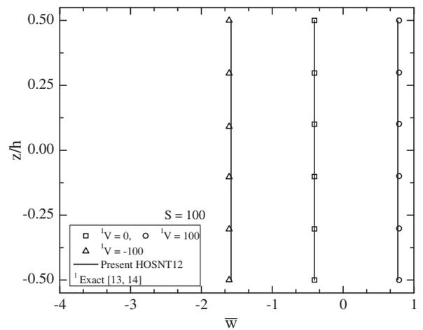
**Fig. 3.** Variation of normalized transverse displacement ( $\bar{w}$ ) through the thickness of symmetric substrate ( $0^\circ/90^\circ/0^\circ$ ) without and with applied sinusoidal electric voltages at top of the PFRC actuator surface.
