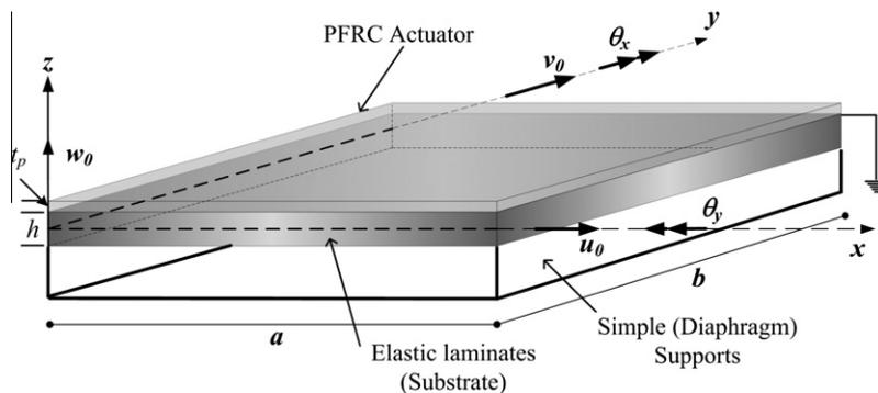
Fig. 1. Geometry of elastic substrate simply (diaphragm) supported along all edges attached with PFRC actuator at top.
