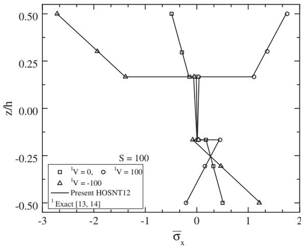
**Fig. 4.** Variation of normalized in-plane normal stress ( $\bar{\sigma}_x$ ) through the thickness of symmetric substrate ( $0^\circ/90^\circ/0^\circ$ ) without and with applied sinusoidal electric voltages at top of the PFRC actuator surface.
