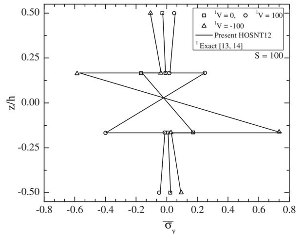
**Fig. 5.** Variation of normalized in-plane normal stress ( $\bar{\sigma}_y$ ) through the thickness of symmetric substrate ( $0^\circ/90^\circ/0^\circ$ ) without and with applied sinusoidal electric voltages at top of the PFRC actuator surface.
