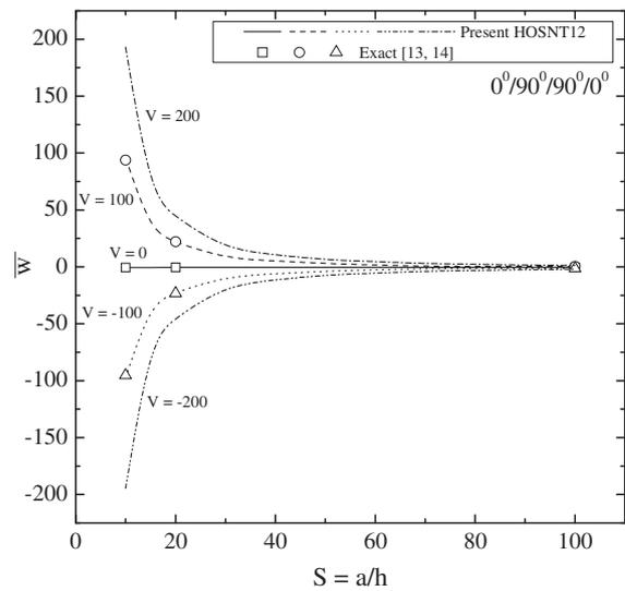
**Fig. 9.** Variation of normalized transverse displacement ( $\bar{w}$ ) with respect to aspect ratio ( $S = a/h$ ) of symmetric substrate ( $0^\circ/90^\circ/90^\circ/0^\circ$ ) without and with applied sinusoidal electric voltages at top of the PFRC actuator surface.
