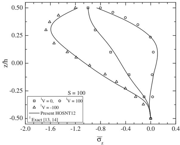
**Fig. 6.** Variation of normalized transverse normal stress ( $\bar{\sigma}_z$ ) through the thickness of symmetric substrate ( $0^\circ/90^\circ/0^\circ$ ) without and with applied sinusoidal electric voltages at top of the PFRC actuator surface.
