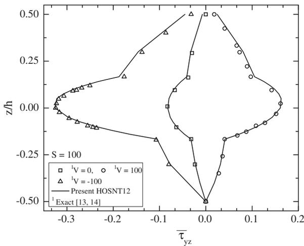
**Fig. 8.** Variation of normalized transverse shear stress ( $\bar{\tau}_{yz}$ ) through the thickness of symmetric substrate ( $0^\circ/90^\circ/0^\circ$ ) without and with applied sinusoidal electric voltages at top of the PFRC actuator surface.
