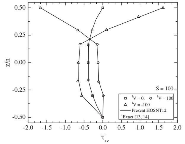
**Fig. 7.** Variation of normalized transverse shear stress ( $\bar{\tau}_{xz}$ ) through the thickness of symmetric substrate ( $0^\circ/90^\circ/0^\circ$ ) without and with applied sinusoidal electric voltages at top of the PFRC actuator surface.
