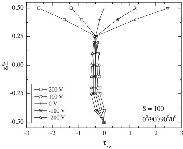
**Fig. 10.** Normalized transverse shear stress ( $\tau_{xz}$ ) across the thickness of symmetric substrate ( $0^\circ/90^\circ/90^\circ/0^\circ$ ) without and with applied sinusoidal electric voltages at top of the PFRC actuator surface.
