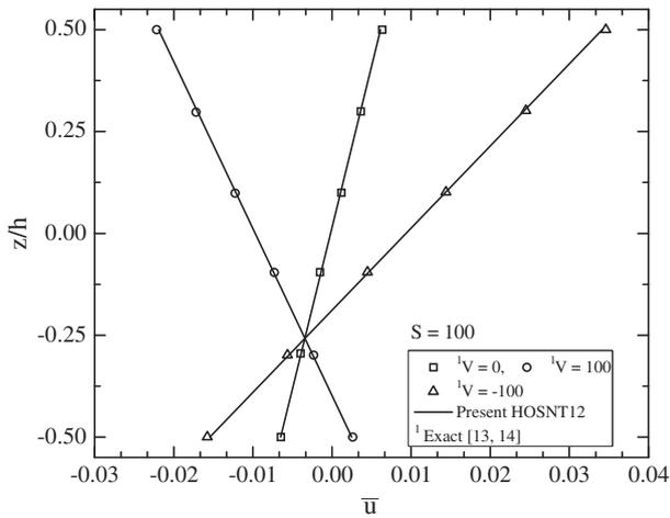
**Fig. 2.** Variation of normalized in-plane displacement ( $\bar{u}$ ) through the thickness of symmetric substrate ( $0^\circ/90^\circ/0^\circ$ ) without and with applied sinusoidal electric voltages at top of the PFRC actuator surface.
