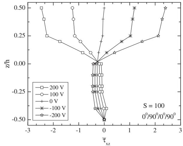
**Fig. 11.** Normalized transverse shear stress ( $\tau_{xz}$ ) across the thickness of antisymmetric substrate ( $0^\circ/90^\circ/0^\circ/90^\circ$ ) without and with applied sinusoidal electric voltages at top of the PFRC actuator surface.
