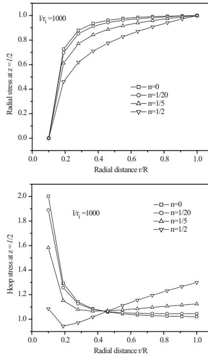
Fig. 7 Comparison of radial and hoop stress through thickness with different non-homogeneity parameters for  $r_i/r_o = 1/10$  and for  $l/r_i = 1000$  under pressure loading.
