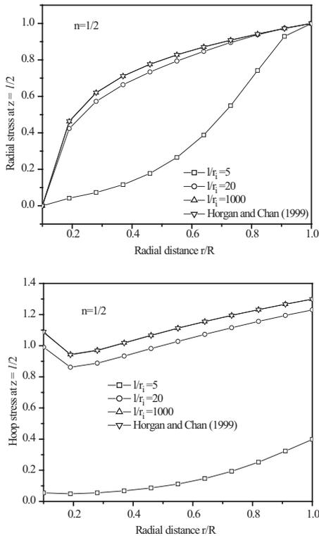
Fig. 5 Distribution of radial and hoop stress through thickness for  $n=1/2$  and  $r_i/r_o = 1/10$  under pressure loading.
