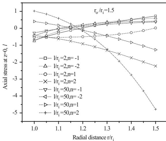
Fig. 14 Distribution of axial stress  $\overline{\sigma_z}$  through thickness for functionally graded thick cylinder under thermal loading.
