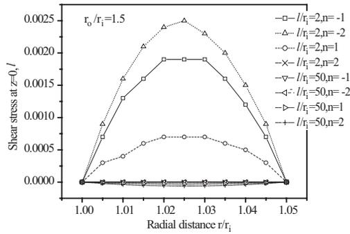
Fig. 18 Distribution of shear stress  $\overline{\tau_{rz}}$  through thickness for functionally graded thin cylinder under thermal loading.
