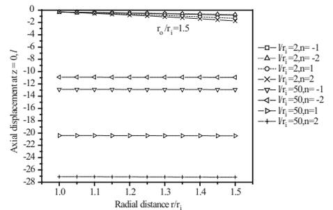
Fig. 10 Distribution of axial displacement  $\bar{w}$  through thickness for functionally graded thick cylinder under thermal loading.
