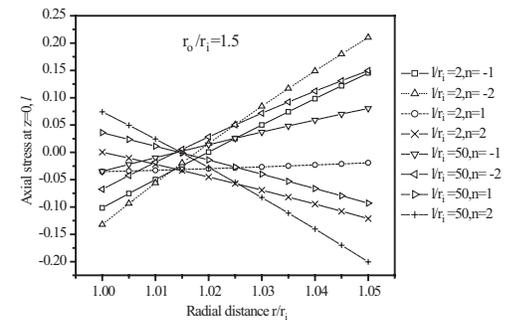
Fig. 20 Distribution of axial stress  $\overline{\sigma_z}$  through thickness for functionally graded thin cylinder under thermal loading.
