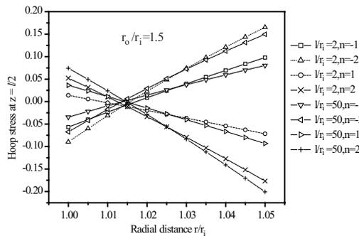
Fig. 19 Distribution of hoop stress  $\overline{\sigma_{\theta}}$  through thickness for functionally graded thin cylinder under thermal loading
