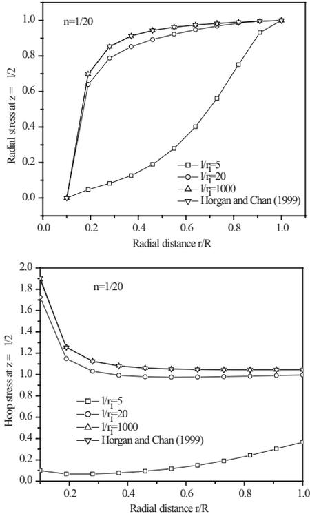
Fig. 4 Distribution of radial and hoop stress through thickness for  $n=1/20$  and  $r_i/r_o = 1/10$  under pressure loading.
