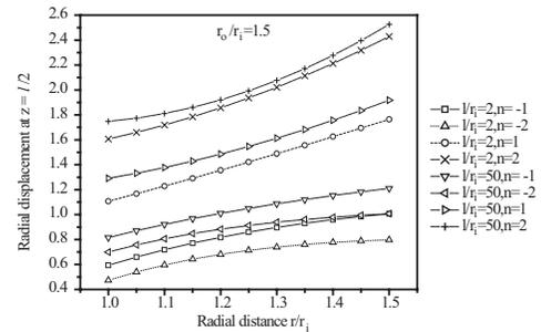
Fig. 9 Distribution of radial displacement  $\bar{u}$  through thickness for functionally graded thick cylinder under thermal loading.
