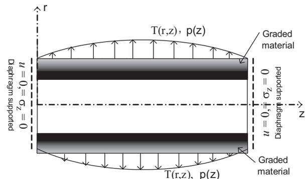
Fig. 1b Finite FG cylinder under sinusoidal external thermal and pressure loading
