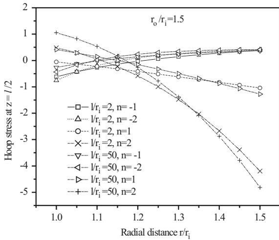
Fig. 13 Distribution of hoop stress  $\overline{\sigma_{\theta}}$  through thickness for functionally graded thick cylinder under thermal loading.
