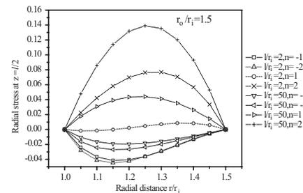
Fig. 11 Distribution of radial stress  $\bar{\sigma}_r$  through thickness for functionally graded thick cylinder under thermal loading.
