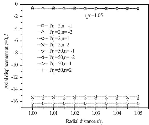
Fig. 16 Distribution of axial displacement  $\overline{w}$  through thickness for functionally graded thin cylinder under thermal loading.
