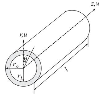
Fig. 1a Coordinate system and geometry of cylinder
