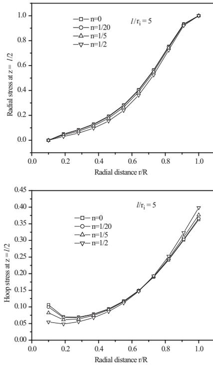
Fig. 8 Comparison of radial and hoop stress through thickness with different non-homogeneity parameters for  $r_o/r_i = 1/10$  for  $l/r_i = 5$  under pressure loading.
