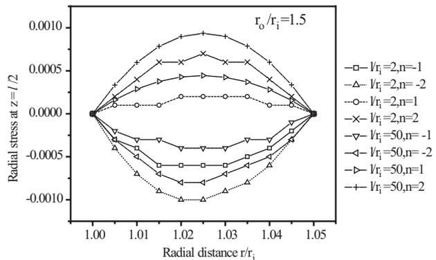
Fig. 17 Distribution of radial stress  $\overline{\sigma_r}$  through thickness for functionally graded thin cylinder under thermal loading.
