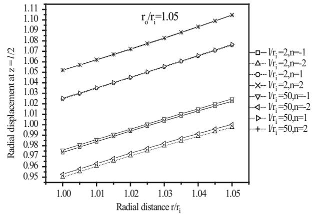
Fig. 15 Distribution of radial displacement  $\overline{u}$  through thickness for functionally graded thin cylinder under thermal loading.
