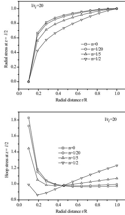
Fig. 6 Comparison of radial and hoop stress through thickness with different non-homogeneity parameters for  $r_i/r_o = 1/10$  and  $l/r_i = 20$  under pressure loading.
