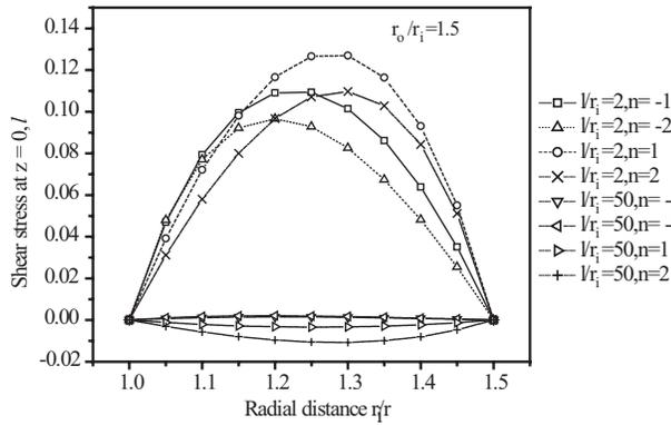
Fig. 12 Distribution of shear stress  $\overline{\tau_{rz}}$  through thickness for functionally graded thick cylinder under thermal loading
